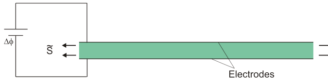
Figure 6.2: A specimen is prestressed and activated electrically at S_{11} = \tilde{S} , applying a constant force \tilde{S} along x_2 direction.
