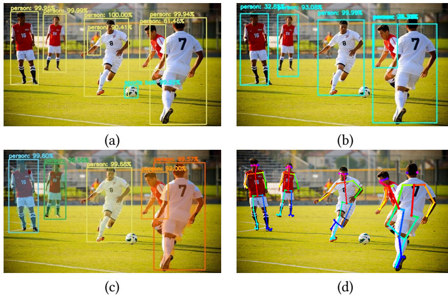
Figure 6.7: An example of application of YOLO (a), SSD (b), Mask R-CNN (c) and OpenPose (d) applied on the same image.
