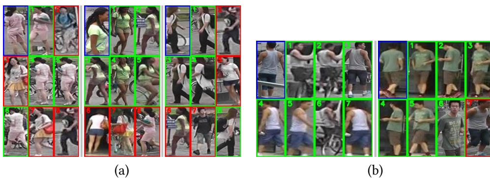
Figure 6.9: KNN applied to images elaborated with 11 real people and ResNet50 (a) and with 2 real people and GoogLeNet (b), with 9 images of each person. The query (images with the blue contour) is used to extract from the database the most similar pre-analysed images. The green contour depicts the correct extracted person, whereas the red contour highlights wrongly extracted persons.
