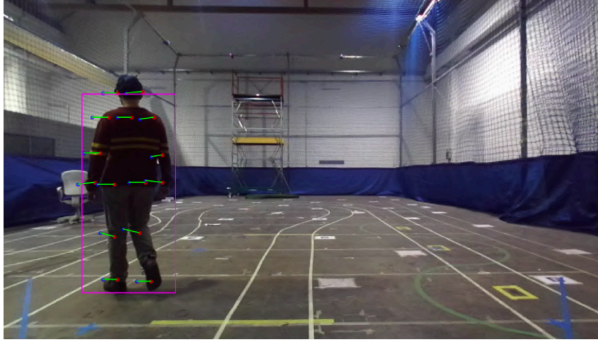
Figure 3.5: Human detected with OpenPose (blue and red points) and with YOLO (purple box).
