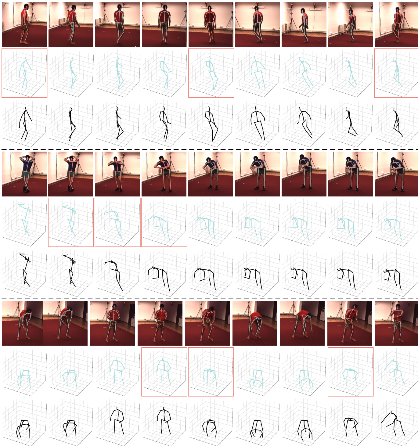
Fig. 10: Visualization of input images, estimated 3D poses (cyan), and ground truth 3D poses (black) from three video sequences. The 2D poses of selected frames are colored in red, and the 2D poses of pruned frames are colored in gray. The 3D poses of selected frames are highlighted with red rectangular boxes.
