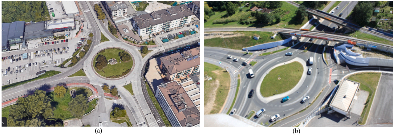
Fig.3. Roundabouts considered for the model calibration a) conventional roundabout in Trento (Italy); b) basic turbo roundabout in Maribor (Slovenia).
