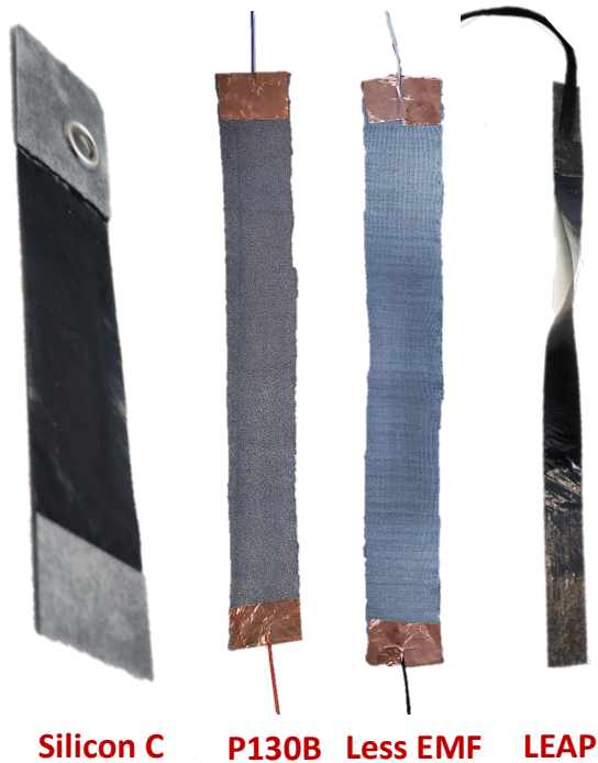
Figure 5-1: Different stretch sensors studied to be used in an active soft brace.
