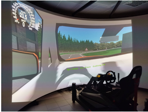
FIGURE 25. The driving Simulator of the University of Trento uses a 3 degrees of freedom platform that reproduces heave, pitch, and roll motion in an immersive wide screen.
