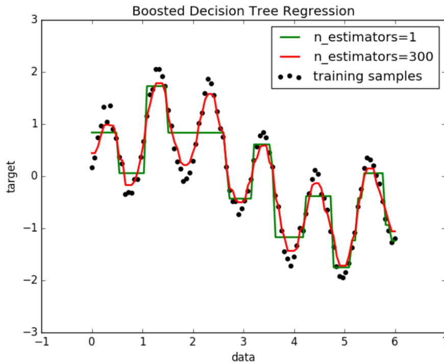
Figure 1.23: Boosting method for decision tree regression with 2 values of the hyperparameter n\_estimators ( https://scikit-learn.org/stable/auto_examples/ensemble/plot_adaboost_regression.html ).
