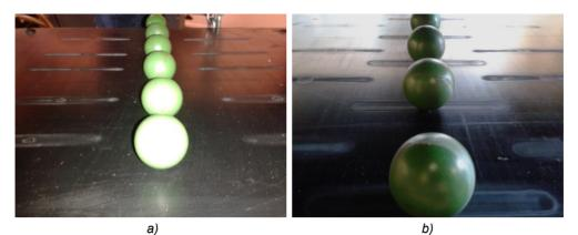
Fig. 6.60 Semi-permanent rolling tracks on the rubber layer B. Case B-B,  $t_{dw}$ =24 h, W=250 N: a) before the test (the semi-permanent rolling tracks visible derive from the previous test with W=150 N); b) afer the test.
