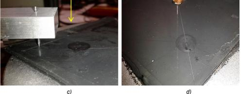
Fig. 6.36 Details of the setup (a) for the measurement of the pit profiles: b) non-contacting capacitance probe and c) needle probe at the two ends of the aluminium alloy bar. d) View of a pit after some measures (the lines shown the measurement directions).
