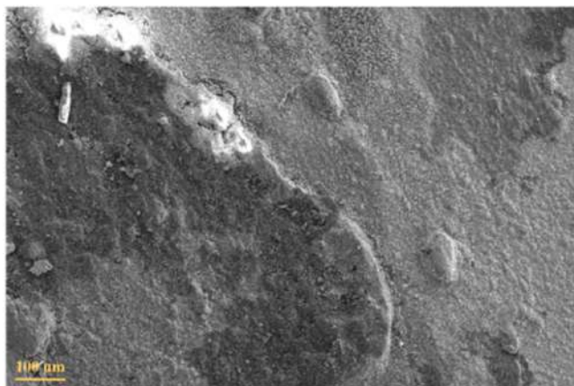
Fig. 18. FESEM image of corroded MS sample.
