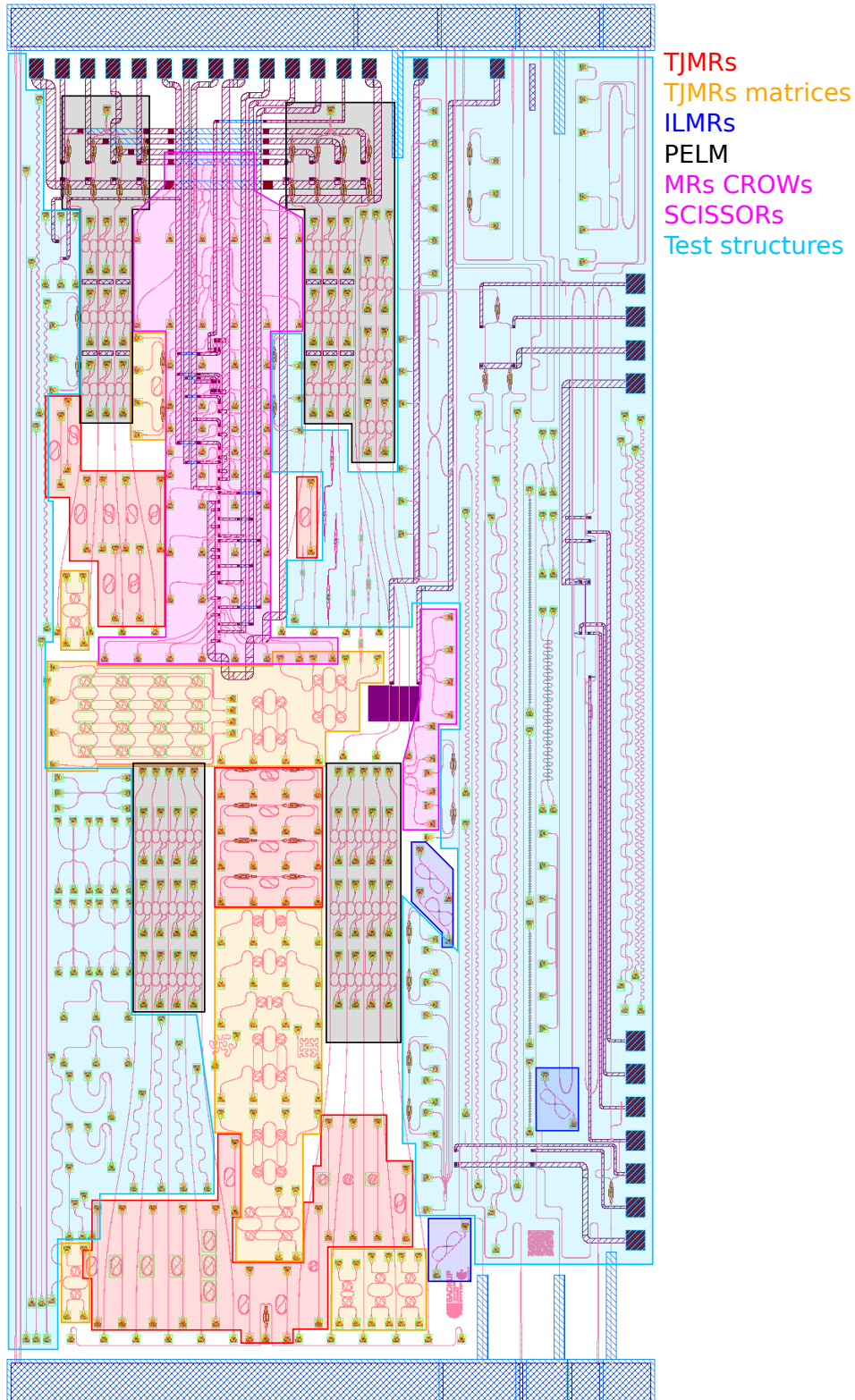
Figure A.1: Design of the Mask2020 chip. Red boxes highlight the TJMRs, the orange boxes the TJMRs matrices, the blue ones the ILMRs, the black ones the PELM structures, the fuchsia ones the microring resonators, the side-coupled integrated sequences of resonators (SCISSORs) and coupled resonators optical waveguides (CROWs) and lastly the cyan boxes highlight the test structures.
