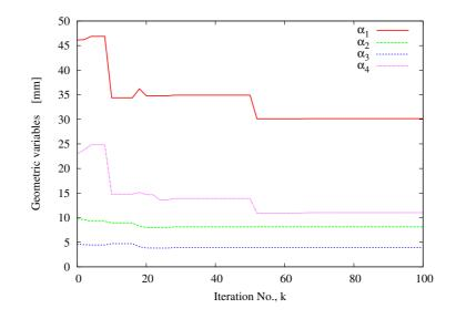
Figure 4.7: Test Case A - Evolution of the geometric variables  $\{\alpha_1, ..., \alpha_4\}$  over the iterations.
