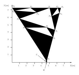
Figure 5.7: Geometry of the multimode three-band antenna.
