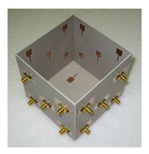
Figure 7.12: Prototype of the 24-element array.
