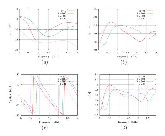
Figure 3.6: Optimization Process Analysis - Parametric Approach - Plot of (a)  $|s_{11}|$ , (b)  $|s_{21}|$ , (c)  $\angle s_{21}$ , and (d)  $\tau$  versus the frequency at different iterations of the optimization process.
