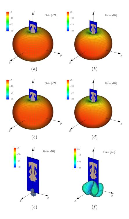
Figure 5.18: Simulated 3D radiation patterns - Total gain at (a)  $f_1 = 2.448 GHz$ and (b)  $f_2 = 5.512 GHz$ . Co-polar component at (c)  $f_1 = 2.448 GHz$  and (d)  $f_2 = 5.512 GHz$ . Cross-polar component at (e)  $f_1 = 2.448 GHz$  and (f)  $f_2 = 5.512 GHz$ .
