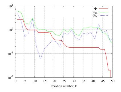
Figure 5.8: Behaviors of the cost function statistics during the iterative PSO optimization.
