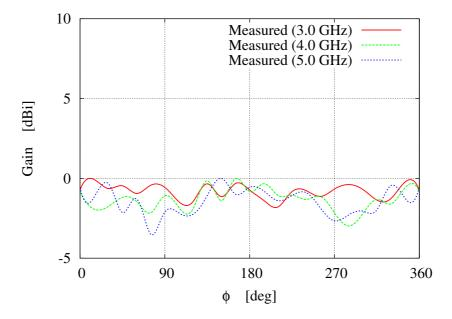
Figure 3.14: UWB Dongle Antenna - Measured H-plane radiation pattern.
