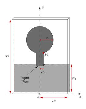
Figure 3.4: *Optimization Process Analysis - Parametric approach* - Descriptive parameters for the circular monopole reference geometry.
