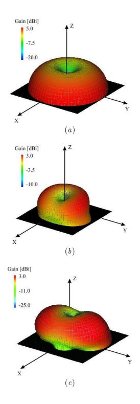
Figure 5.12: Simulated 3D radiation patterns - (a) Total gain at  $f_0^{DVBH} = 610 MHz$ ; (b) Total gain at  $f_0^{GSM1800} = 1850 MHz$ ; (c) Total gain at  $f_0^{UMTS} = 2100 MHz$ .
