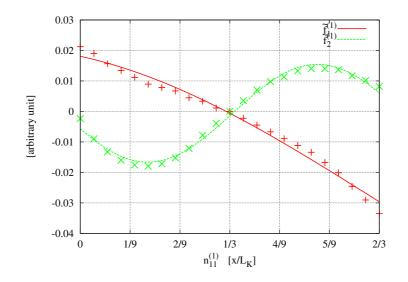
Figure 5.4: *Perturbation analysis*. Behavior of the normalized resonant frequencies of the Koch antenna varying the  $n_{11}^{(1)}$  parameter.
