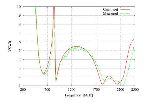
Figure 5.11: Simulated and measured VSWR values.
