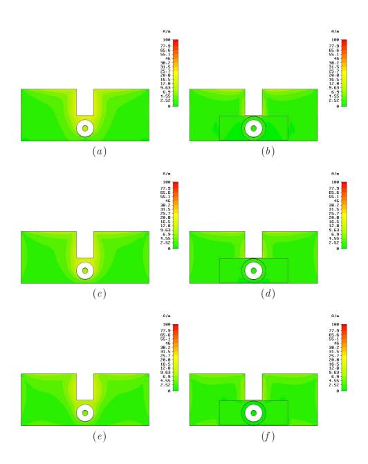
Figure 7.5: Surface currents flowing on the groundplane of the synthesized antenna element. (a)(c)(e) Front and (b)(d)(f) back side at (a)(b) 2.5, (c)(d) 4.0, and (e)(f) 5.5 GHz.
