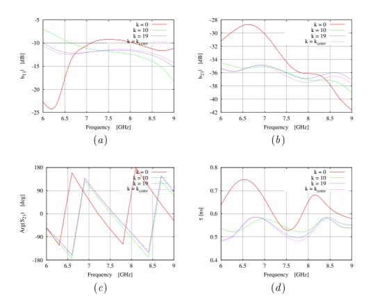
Figure 3.3: Optimization Process Analysis - Plot of (a)  $|s_{11}|$ , (b)  $|s_{21}|$ , (c)  $\angle s_{21}$ , and (d)  $\tau$  versus the frequency at different iterations of the optimization process.
