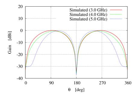
Figure 3.16: UWB Dongle Antenna - Simulated E-plane radiation pattern ( $\phi = 90^{\circ}$ ).
