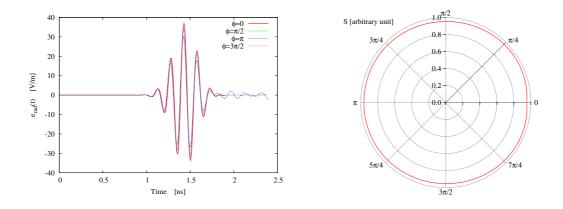
Figure 4.12: Test Case A - Radiated electric field towards different directions and corresponding similarity factor values.
