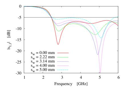
Figure 7.9: Simulated  $s_{1,1}$  magnitude values exhibited by the antenna for different values of the slit width  $s_w$ .
