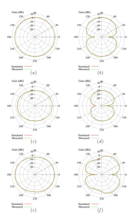
Figure 3.30: Band Notched Antenna - Behavior of the absolute gain at (a)-(b) $f_1 = 4 \,GHz$ , (c)- $(d) f_{notch} = 5.25 \,GHz$ , and (e)- $(f) f_2 = 8 \,GHz$  along (a)(c)(e) the horizontal  $(\theta = 90^\circ)$  and (b)(d)(f) the vertical plane  $(\phi = 90^\circ)$ .
