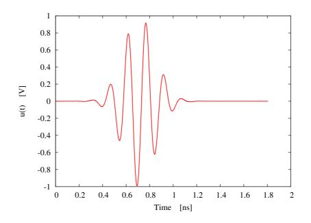
Figure 4.6: Test Case A - Time domain behavior of the input signal u(t).
