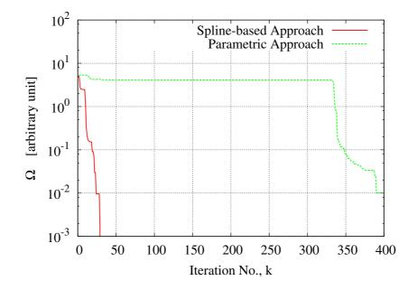
Figure 3.7: Optimization Process Analysis - Comparison between parametric approach and spline-based approach - Plot of the optimal value of the cost function  $\Omega$  and corresponding terms versus the iteration number k.
