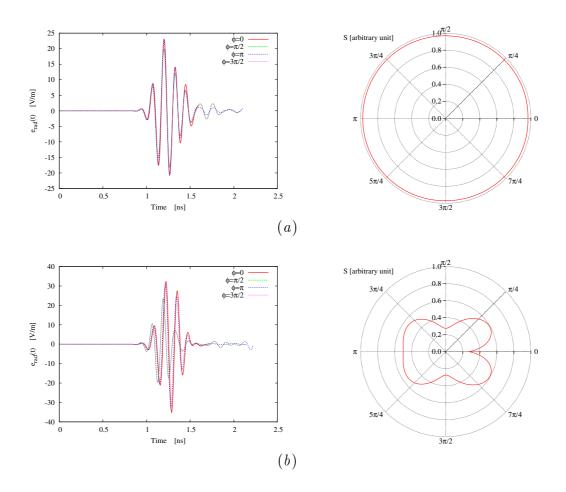
Figure 4.4: Similarity Factor - Examples of radiated electric field towards different directions and the corresponding similarity factor values. (a)  $0.9 < S(\theta, \phi) < 1$  and (b)  $0.2 < S(\theta, \phi) < 0.6$ .
