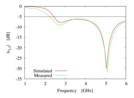
Figure 7.3: Simulated and measured  $s_{1,1}$  magnitude values exhibited by the synthesized antenna element.
