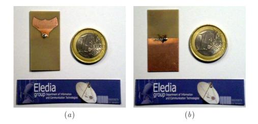
Figure 3.9: UWB Dongle Antenna - (a) Front view and (b) back view of the antenna prototype.
