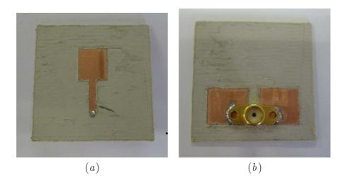
Figure 7.2: Prototype of the synthesized antenna element. (a) Front view and (b) back view.
