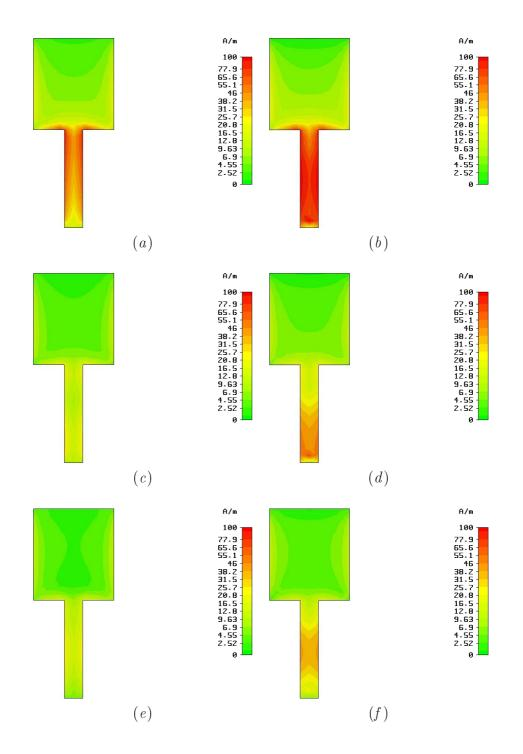
Figure 7.6: Surface currents flowing on the feedline and the patch of the modified antenna element (without the slit). (a)(c)(e) Front and (b)(d)(f) back side at (a)(b) 2.5, (c)(d) 4.0, and (e)(f) 5.5 GHz.
