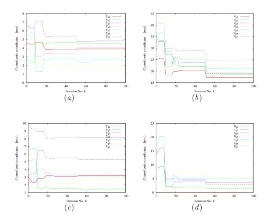
Figure 4.8: Test Case A - Evolution of the coordinates of the control points of the splines modeling (a) the radiating part and (b) the ground plane of the antenna over the iterations.
