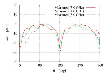
Figure 3.18: UWB Dongle Antenna - Measured E-plane radiation pattern ( $\phi = 90^{\circ}$ ).
