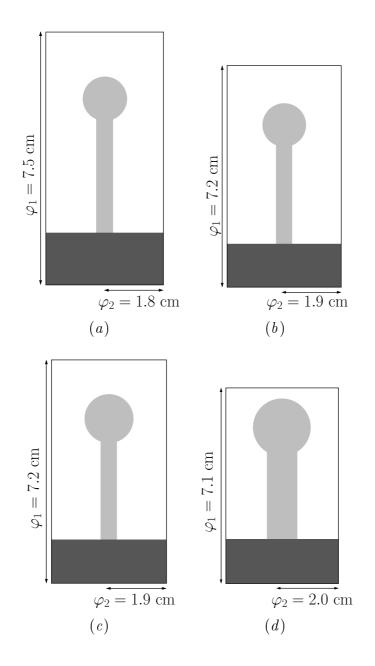
Figure 3.5: Optimization Process Analysis - Parametric Approach - Evolution of the antenna shape: (a) k = 0, (b) k = 100, (c) k = 300, and (d) k = K = 400.
