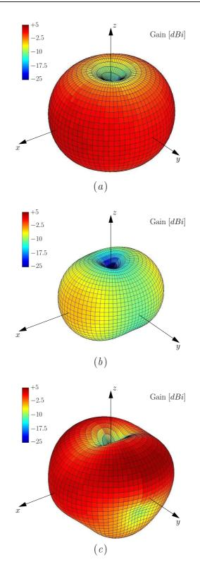
Figure 3.29: Band Notched Antenna - Three-dimensional representation of the absolute gain pattern at (a)  $f_1 = 4 GHz$ , (b)  $f_{notch} = 5.25 GHz$ , and (c)  $f_2 = 8 GHz$ .
