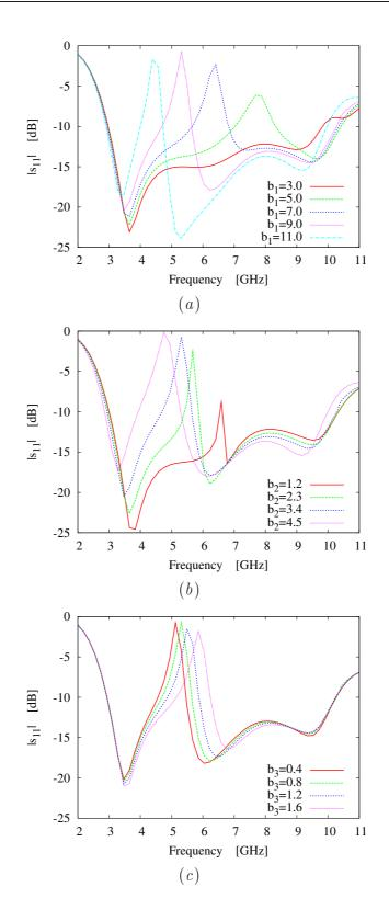
Figure 3.28: Band Notched Antenna - Behavior of the magnitude of  $s_{11}$  varying the parameters (a)  $b_1$ , (b)  $b_2$ , and (c)  $b_3$  describing the slot.
