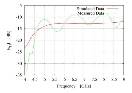
Figure 3.19: FCC Compliant Antenna - Comparison between simulated and measured  $s_{11}$  amplitude values.
