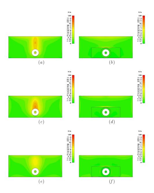
Figure 7.7: Surface currents flowing on the groundplane of the modified antenna element (without the slit). (a)(c)(e) Front and (b)(d)(f) back side at (a)(b) 2.5, (c)(d) 4.0, and (e)(f) 5.5 GHz.
