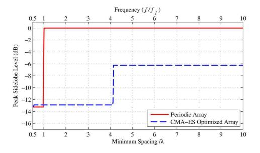
Figure 6.8: Peak sidelobe level performances over an extended bandwidth of the optimized array and of a periodic array populated by the same number of elements.
