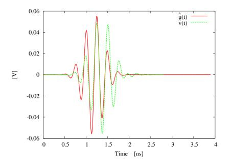
Figure 4.19: Test Case B - Comparison between the energy-normalized input signal  $\hat{u}(t)$  and the energy normalized received signal  $\hat{v}(t)$ .
