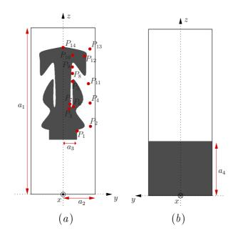
Figure 5.15: Antenna geometry - (a) Front view and (b) back view.
