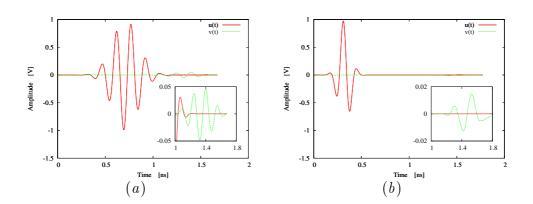
Figure 4.3: System Fidelity - Examples of transmitted and received signals giving (a) F = 0.9 and (b) F = 0.5.
