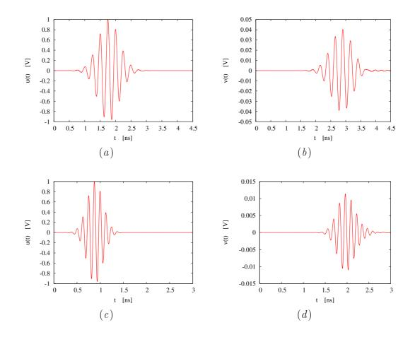
Figure 3.32: Band Notched Antenna - Transmitted (a)(c) and received (b)(d) pulses at the frequency bands (a)(b) 3-5 GHz and (c)(d) 6-10 GHz of the UWB system composed of two identical face-to-face copies of the proposed antenna.
