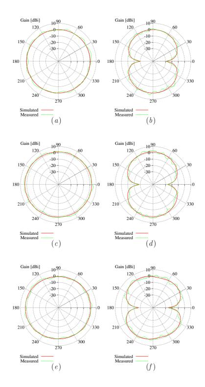
Figure 4.16: Test Case A - Comparison between simulated and measured values of total gain at (a)-(b) 4 GHz, (c)-(d) 6.5 GHz, and (e)-(f) 9 GHz in the (a)-(c)-(e) horizontal  $(\theta = 90^{\circ})$  and (b)-(d)-(f) vertical plane  $(\phi = 90^{\circ})$ .
