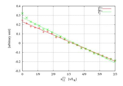
Figure 5.5: *Perturbation analysis*. Behavior of the normalized resonant frequencies of the Koch antenna varying the  $n_{12}^{(1)}$  parameter.
