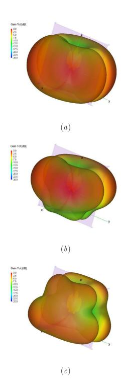
Figure 6.6: Three-dimensional representation of the total gain pattern at (a) 2, (b) 4 and (c) 6 GHz.
