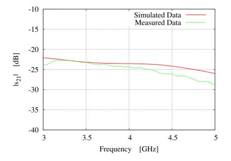
Figure 3.11: UWB Dongle Antenna - Amplitude of  $s_{21}$  vs. frequency.
