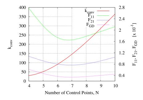
Figure 3.8: Optimization Process Analysis - Behavior of the quality indexes  $F_{11}$ ,  $F_{21}$ ,  $F_{GD}$  and of  $k_{conv}$  versus the number of control points N.
