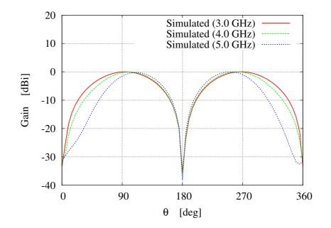
Figure 3.15: UWB Dongle Antenna - Simulated E-plane radiation pattern ( $\phi = 0^{\circ}$ ).
