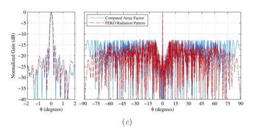
Figure 6.10: Comparison between the normalized power pattern and the array factor of the array at (a) 2, (b) 4 and (c) 6 GHz.
