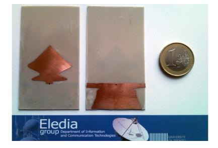
Figure 4.17: Test Case B - Antenna prototype.
