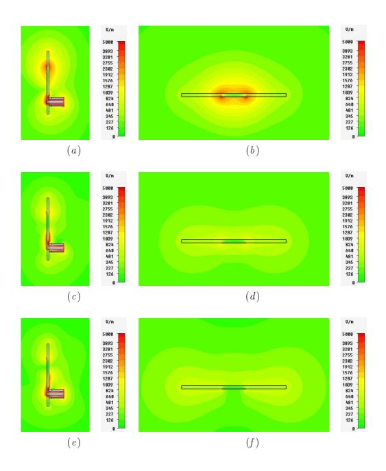
Figure 7.10: Electric near field radiated by the synthesized antenna. (a)(c)(e)Vertical and (b)(d)(f) horizontal plane passing by the center of the rectangular patch at (a)(b) 2.5, (c)(d) 4.0, and (e)(f) 5.5 GHz.
