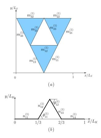
Figure 5.1: Fractal antenna geometries considered in the perturbation analysis. (a) Sierpinski antenna and (b) Koch antenna.
