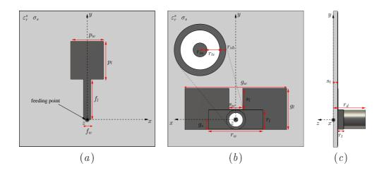
Figure 7.1: Geometry of the printed rectangular monopole antenna. (a) Front view, (b) back view and (c) side view.
