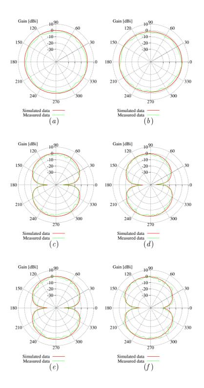
Figure 5.19: Simulated and measured radiation patterns - Horizontal plane ( $\theta = 90^{\circ}$ ) at (a)  $f_1 = 2.448 \, GHz$  and (b)  $f_2 = 5.512 \, GHz$ . Vertical plane ( $\phi = 0^{\circ}$ ) at (c)  $f_1 = 2.448 \, GHz$  and (d)  $f_2 = 5.512 \, GHz$ . Vertical plane ( $\phi = 90^{\circ}$ ) at (e)  $f_1 = 2.448 \, GHz$  and (f)  $f_2 = 5.512 \, GHz$ .
