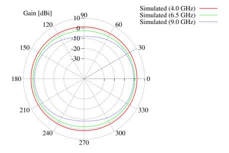
Figure 3.22: FCC Compliant Antenna - Radiation patterns in the horizontal plane.
