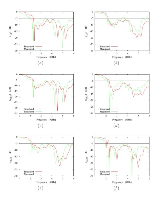
Figure 7.13: Simulated and measured return loss values exhibited by the array elements. (a)  $|s_{1,1}|$ , (b)  $|s_{3,3}|$ , (c)  $|s_{11,11}|$ , (d)  $|s_{14,14}|$ , (e)  $|s_{18,18}|$ , and (f)  $|s_{22,22}|$ .
