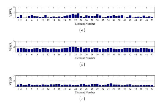
Figure 6.9: VSWR values for all the elements of the array at (a) 2, (b) 4 and (c) 6 GHz.
