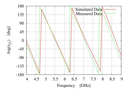
Figure 3.21: FCC Compliant Antenna - Comparison between simulated and measured  $s_{21}$  amplitude values.
