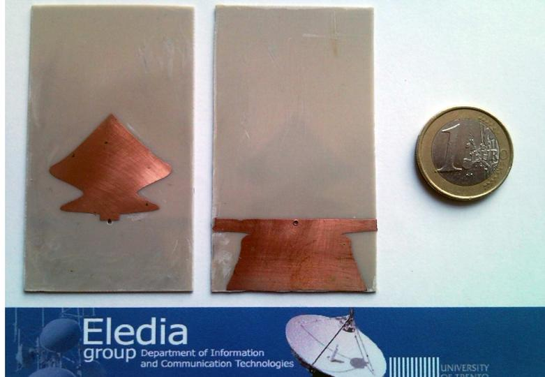
Figure 4.17: *Test Case B* - Antenna prototype.
