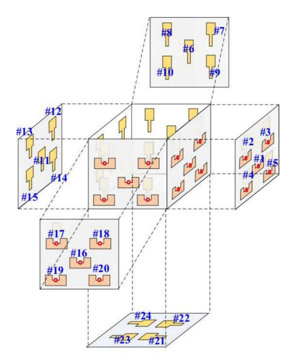
Figure 7.11: Layout of the 24-element array.
