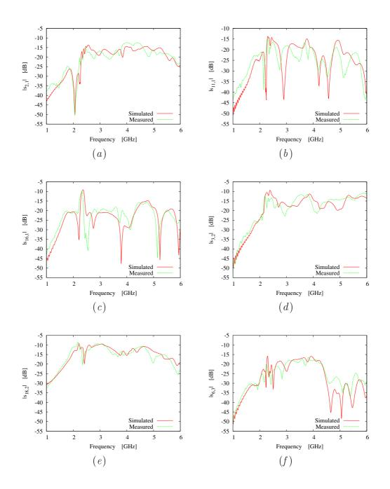
Figure 7.14: Simulated and measured transmission coefficient values exhibited by the array elements. (a)  $|s_{2,1}|$ , (b)  $|s_{11,1}|$ , (c)  $|s_{16,1}|$ , (d)  $|s_{3,2}|$ , (e)  $|s_{18,2}|$ , and (f)  $|s_{6,3}|$ .
