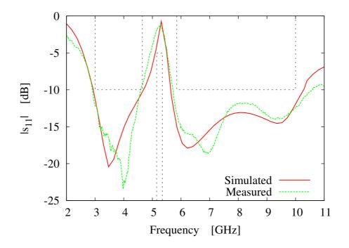
Figure 3.26: Band Notched Antenna - Behavior of the magnitude of  $s_{11}$  within the UWB frequency range.
