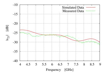
Figure 3.20: FCC Compliant Antenna - Comparison between simulated and measured  $s_{21}$  amplitude values.
