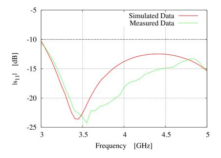
Figure 3.10: UWB Dongle Antenna - Amplitude of  $s_{11}$  vs. frequency.
