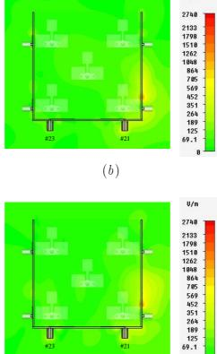
Figure 7.17: Electric near field radiated by the array antenna #4 on the vertical plane passing by the center of the antenna #21 rectangular patch at (a) 2.5, (b) 4.0, and (c) 5.5 GHz.
