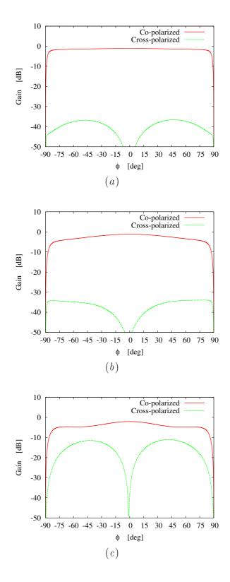
Figure 6.7: Behavior of the co-polarized and cross-polarized gain components in the plane of  $\theta = \frac{\pi}{2}$  at (a) 2, (b) 4 and (c) 6 GHz.
