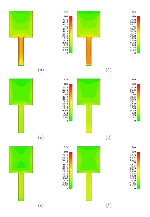
Figure 7.4: Surface currents flowing on the feedline and the patch of the synthesized antenna element. (a)(c)(e) Front and (b)(d)(f) back side at (a)(b) 2.5, (c)(d) 4.0, and (e)(f) 5.5 GHz.
