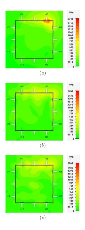
Figure 7.15: Electric near field radiated by the array antenna #4 on the horizontal plane passing by the center of the rectangular patch at (a) 2.5, (b) 4.0, and (c) 5.5 GHz.
