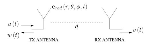
Figure 4.1: UWB communication system composed by a pair of two identical antennas.
