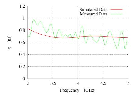
Figure 3.12: UWB Dongle Antenna - Group delay  $\tau_g$  vs. frequency.
