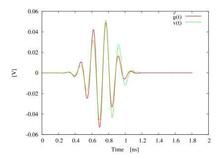
Figure 4.11: Test Case A - Comparison between the energy-normalized input signal  $\hat{u}(t)$  and the energy normalized received signal  $\hat{v}(t)$ .
