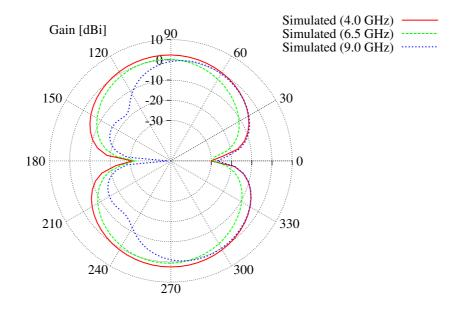
Figure 3.23: FCC Compliant Antenna - Radiation patterns in the  $\phi = 0^{\circ}$  vertical plane.
