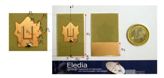
Figure 3.25: *Band Notched Antenna* - Antenna prototype and descriptive parameters.
