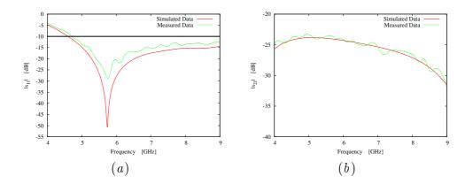
Figure 4.13: Test Case A - Magnitude of (a)  $s_{11}$  and (b)  $s_{21}$  parameters.
