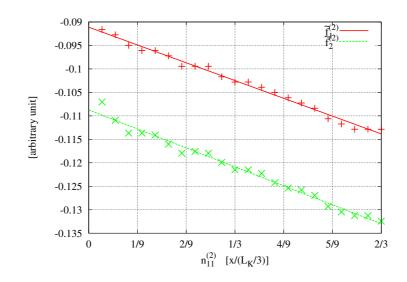
Figure 5.6: *Perturbation analysis*. Behavior of the normalized resonant frequencies of the Koch antenna varying the  $n_{11}^{(2)}$  parameter.
