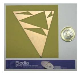
Figure 5.10: Three-band Antenna Prototype.
