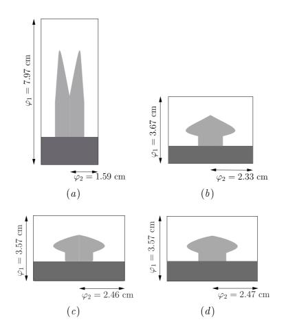
Figure 3.2: Optimization Process Analysis - Evolution of the antenna shape: (a) k = 0, (b) k = 10, (c) k = 19, and (d)  $k = k_{conv} = 28$ .
