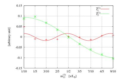
Figure 5.2: *Perturbation analysis*. Behavior of the normalized resonant frequencies of the Sierpinski antenna varying the  $m_{11}^{(1)}$  parameter.
