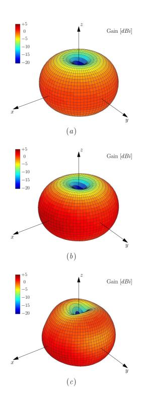
Figure 4.15: Test Case A - Simulated total gain radiation patterns at (a) 4 GHz, (b) 6.5 GHz, and (c) 9 GHz.
