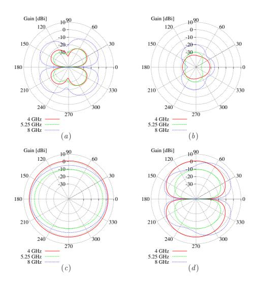
Figure 3.31: Band Notched Antenna - Behavior of the (a)-(b) cross-polar and (c)-(d) co-polar gain components along (a)-(c) the horizontal  $(\theta = 90^{\circ})$  and (b)-(d) the vertical plane  $(\phi = 90^{\circ})$  at  $f_1 = 4 GHz$ ,  $f_{notch} = 5.25 GHz$ , and  $f_2 = 8 GHz$ .
