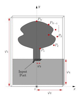
Figure 3.1: Descriptive parameters of the spline-based antenna representation.
