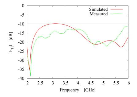
Figure 6.5: Simulated and measured  $s_{11}$  magnitude values exhibited by the synthesized array element.
