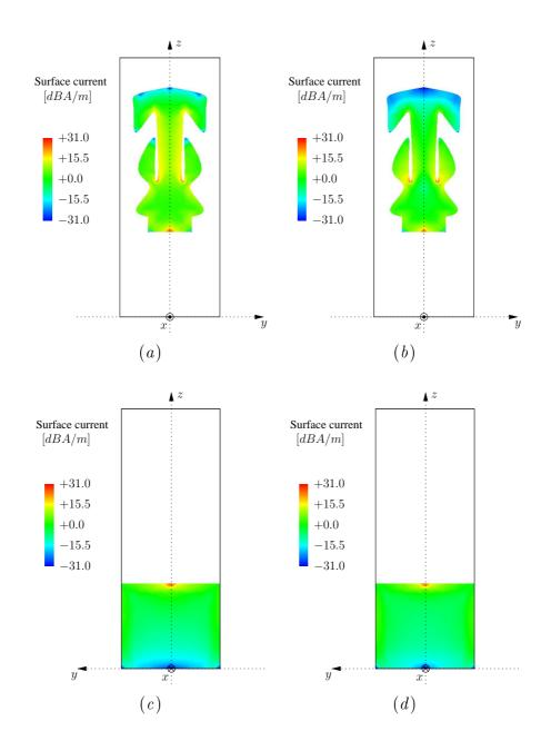
Figure 5.20: Simulated surface current - Front view at (a)  $f_1 = 2.448 GHz$  and (b)  $f_2 = 5.512 GHz$ . Back view at (c)  $f_1 = 2.448 GHz$  and (d)  $f_2 = 5.512 GHz$ .
