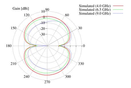
Figure 3.24: FCC Compliant Antenna - Radiation patterns in the  $\phi = 90^{\circ}$  vertical plane.
