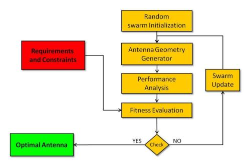
Figure 2.2: PSO-based automatic procedure for the synthesis of an antenna.
