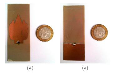
Figure 6.4: Prototype of the synthesized array element. (a) Front view and (b) back view.
