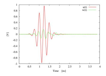
Figure 4.18: Test Case B - Comparison between the input signal u(t) and the reflected signal w(t).
