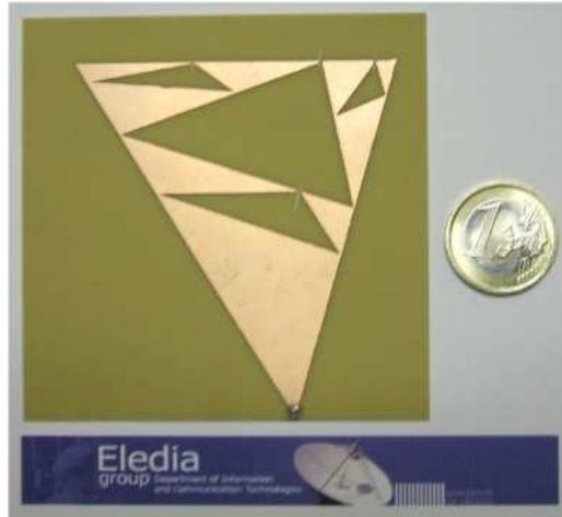
Figure 5.10: Three-band Antenna Prototype.
