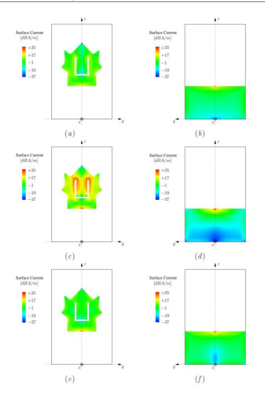
Figure 3.27: Band Notched Antenna - Plots of the surface currents at  $f_1 = 4 GHz$  [(a) Front side and (b) back side],  $f_{notch} = 5.25 GHz$  [(c) Front side and (d) back side], and  $f_2 = 8 GHz$  [(e) Front side and (f) back side].
