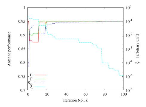
Figure 4.9: Test Case A - Evolution of the antenna performance (antenna efficiency E, system fidelity F, and similarity factor S) over the iterations compared with the cost function  $\xi$ .
