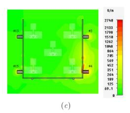
Figure 7.16: Electric near field radiated by the array antenna #4 on the vertical plane passing by the center of the rectangular patch at (a) 2.5, (b) 4.0, and (c) 5.5 GHz.
