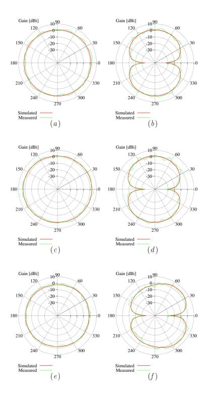
Figure 4.23: Test Case B - Comparison between simulated and measured values of total gain at (a)-(b) 2.5 GHz, (c)-(d) 4 GHz, and (e)-(f) 5.5 GHz in the (a)-(c)-(e) horizontal ( $\theta = 90^{\circ}$ ) and (b)-(d)-(f) vertical plane ( $\phi = 90^{\circ}$ ).
