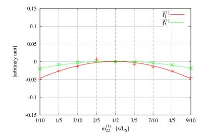
Figure 5.3: *Perturbation analysis*. Behavior of the normalized resonant frequencies of the Sierpinski antenna varying the  $m_{22}^{(1)}$  parameter.
