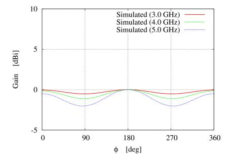
Figure 3.13: UWB Dongle Antenna - Simulated H-plane radiation pattern.
