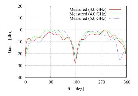
Figure 3.17: UWB Dongle Antenna - Measured E-plane radiation pattern ( $\phi = 0^{\circ}$ ).
