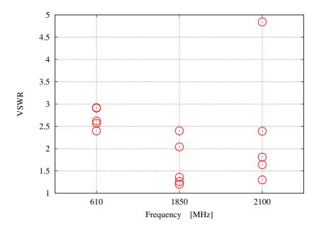
Figure 5.9: Simulated VSWR values, at the center of each frequency band, for the trial solutions at the convergence.
