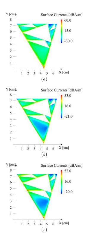
Figure 5.14: Simulated surface currents at (a)  $f_0^{DVBH} = 610 MHz$ , (b)  $f_0^{GSM1800} = 1850 MHz$ , and (c)  $f_0^{UMTS} = 2100 MHz$ .
