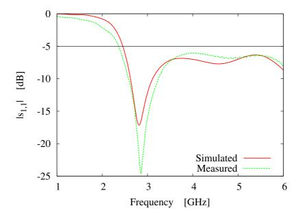
Figure 7.8: Simulated and measured  $s_{1,1}$  magnitude values exhibited by the modified antenna element (without the slit).
