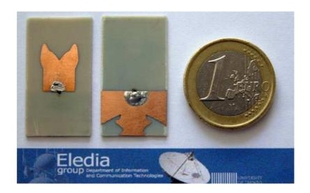
Figure 4.14: Test Case A - Antenna prototype.
