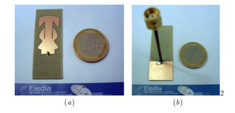
Figure 5.16: Antenna Prototype - (a) Front view and (b) back view.
