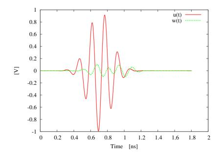
Figure 4.10: Test Case A - Comparison between the input signal u(t) and the reflected signal w(t).
