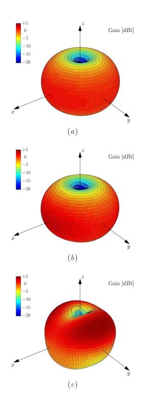
Figure 4.22: Test Case B - Simulated total gain radiation patterns at (a) 2.5 GHz, (b) 4 GHz, and (c) 5.5 GHz.
