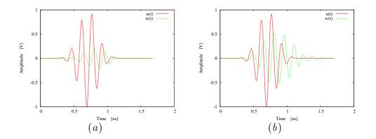
Figure 4.2: Antenna Efficiency - Examples of transmitted and reflected signals giving (a) E = 0.9 and (b) E = 0.5.
