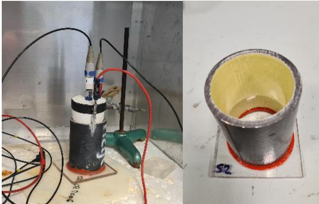
Figure 46 and 47 - Electrochemical cell using a coated pipe cylinder
