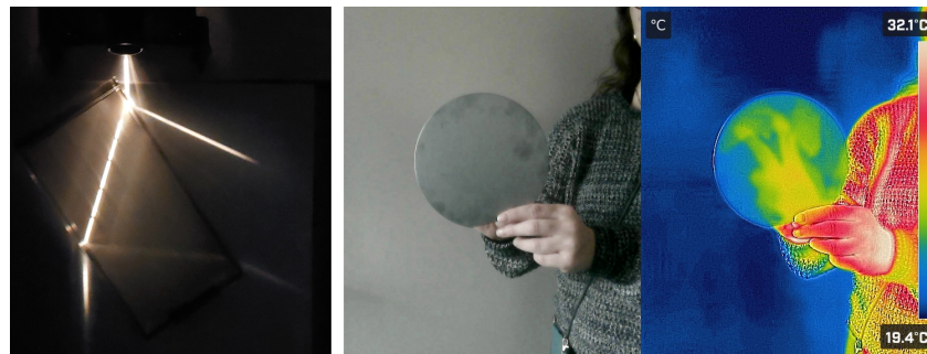
Figure 7. On the left: reflection, refraction, and transmission of a light beam were observed using a rectangular plastic container filled with water. On the right: an infrared image of a student holding a silicon wafer in their hands.
