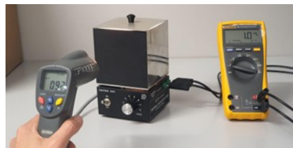
Figure 5. Leslie cube makes it possible to measure the emissivity of different surfaces placed at the same temperature. In fact, the different faces of the cube have significantly different emissivity characteristics.
