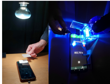
Figure 8. On the left: the desk lamp and the smartphone are positioned less than 10 cm apart, with sheets of paper added one by one above the sensor. On the right: the setup for studying Beer's law of transmittance versus concentration includes a torch with a color filter, a plastic container filled with water, and a smartphone's ambient light sensor to measure light intensity. Drops of color dye are gradually added to the water.
