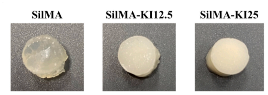
Fig. 2. SilMA and SilMA-KI hydrogels crosslinked by UV rays' exposure.
