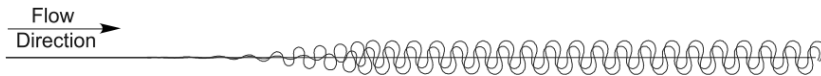
Figure 1.2: Temporal evolution of a meandering planform with convective instability (from Lanzoni and Seminara 2006).
