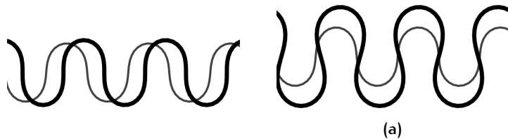
Figure 2.2: Illustrative examples of meander migration modes generated by a periodic mathematical model. (a) Purely downvalley migration. (b) Purely crossvalley migration.
