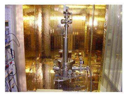
FIGURE 3.4: Torsion pendulum vacuum chamber and the thermal box that surround it.
