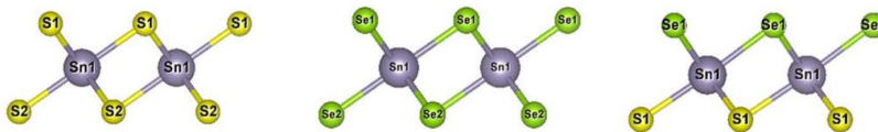
Figure 7.1. Crystal structure of the \text{SnS}_2 , \text{SnSe}_2 , and the Janus \text{SnSSe} monolayer. The atomic structure produced using VESTA software. 194
