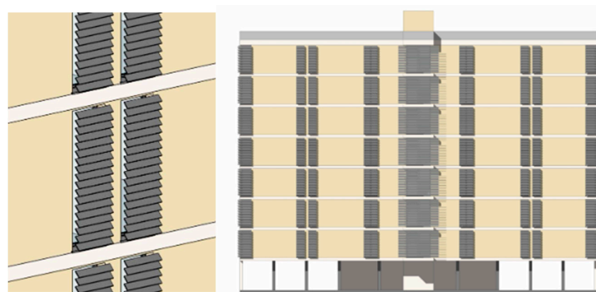
Figure 9. New solar shading elements.
