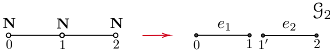
Fig. 2 Model B: on the right, the correct interpretation as a network equation with a disconnected graph
