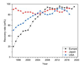
Fig. 5. Recovery rate of ELT from 1994 for Europe, Japan and USA [8,9,50].
