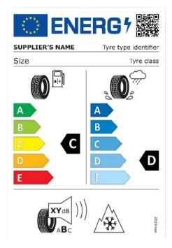
Fig. 2. New EU tyre labelling in accordance with Regulation (EU) 2020/740 [35].
