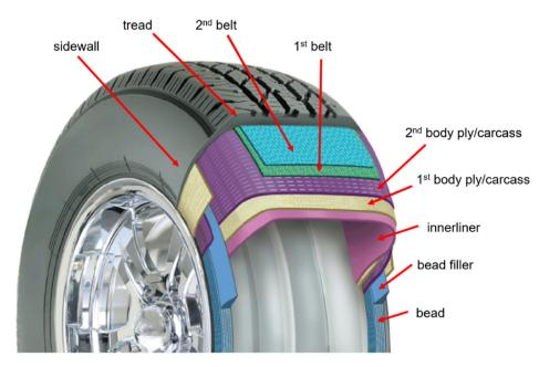
Fig. 1. Exploded view of a commercial passenger car tyre. Adapted from [15].
