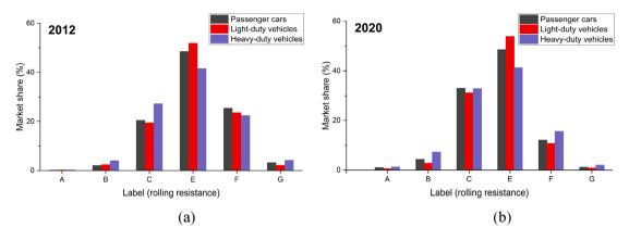
Fig. 3. Market share for passenger car, light-duty vehicle and heavy-duty vehicle tyres in accordance with the EU labelling rules. Comparison between (a) 2012 and (b) 2020 [36].
