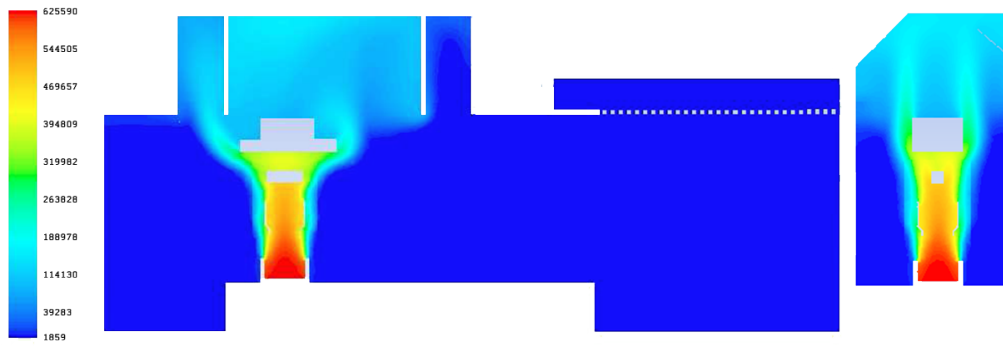
Figure 4.20: Contours of enthalpy (colormap is scaled in J/kg ) calculated with the ideal gas law on the longitudinal (left) and transversal (right) cross sections (without ladle).
