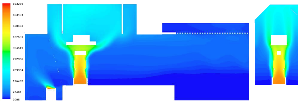
Figure 4.21: Contours of enthalpy (colormap is scaled in J/kg ) in the presence of filled ladle on the longitudinal (left) and transversal (right) cross sections (without ladle).
