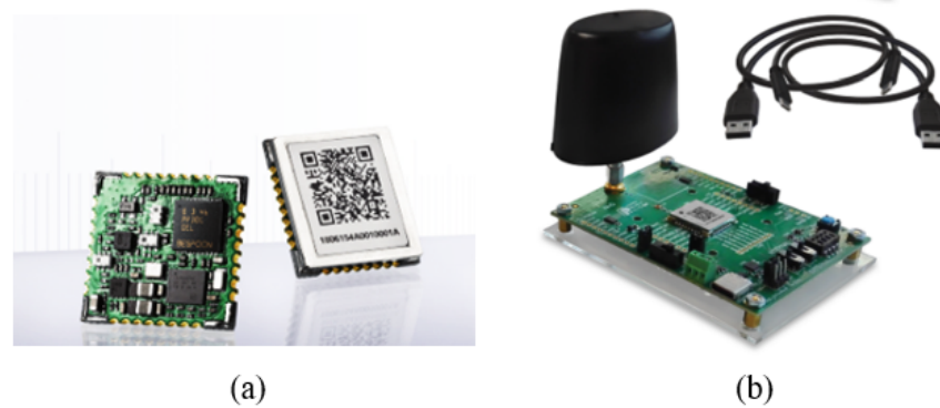
Figure 6. STMicroelectronics: (a) UWB module MOD1 [38], (b) B-UWB-MEK1 application board for MOD1 module with external antenna [42].
