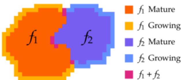
Figure 6: Representation of two different rules evolving together in the Multiple NCA model. Magenta cells are growing cells of both f_1 and f_2 , so they evolve following the average of both rules.
