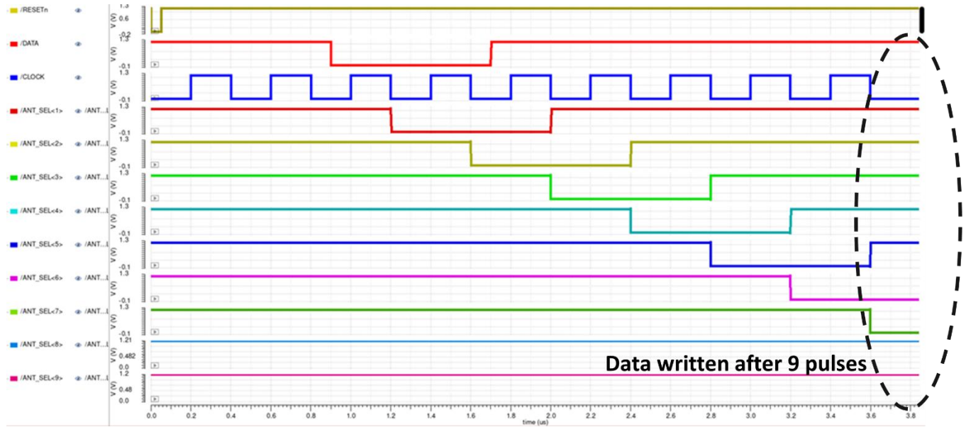
Fig. 4-17. Antenna Selection Shift Register Timing Simulation.
