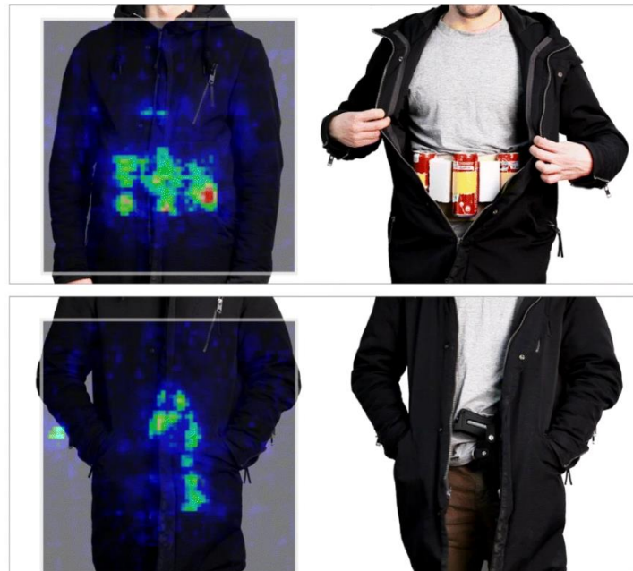
Fig. 1-3. Imaging results showing body-borne concealed threats, a belt with explosives and a gun, obtained by the new sub-THz security body scanner at 3 \mu m range [18].
