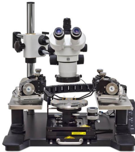
Fig. 3-12. Probe station setup for DC characterization measurements with electrical isolation.
