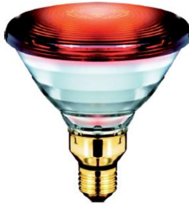
Figure 3. 11. Infrared lamps used in literature to test cool coatings [169–172].
