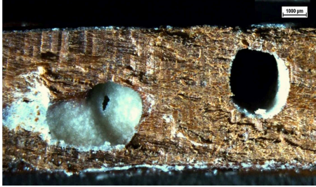
Figure IV- 64. Optical microscope images of long cross-sections of damaged walnut samples untreated (a) and treated with neat Paraloid (b) and microcomposites with 5 wt% and 30 wt% of CMC (c-d).
