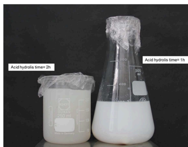
Figure VI- 2. Image of aqueous suspensions of CNC after a sulfuric acid hydrolysis time of 1h and 2h.
