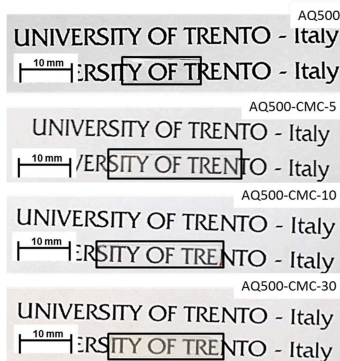
Figure IV- 48. Optical images of thin composite films showing the effect of the addition of 5, 10 and 30 wt% of (a) CNC, (b) CMC on the optical properties of Aquazol 500.
