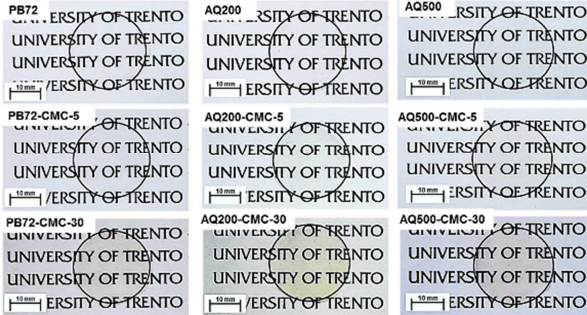
Figure IV- 17. Optical images of thin adhesive composite films showing the effect of the addition of 5 wt% and 30 wt% of CMC on the optical properties of Paraloid and Aquazol matrices.
