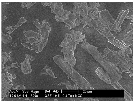
Figure III- 3. ESEM image of cellulose microcrystals.
