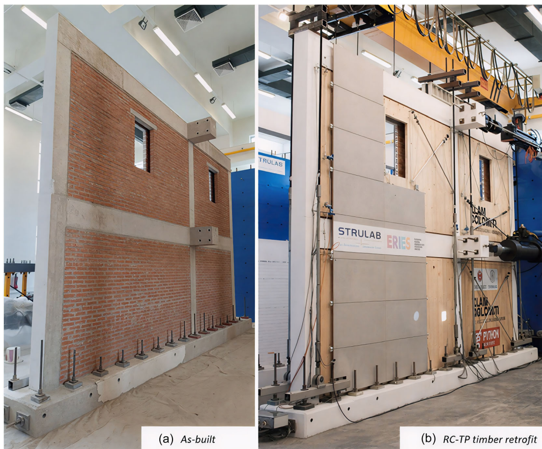
FIGURE 1 | Experimental campaign: full-scale two-storey, two-bay RC frames.
