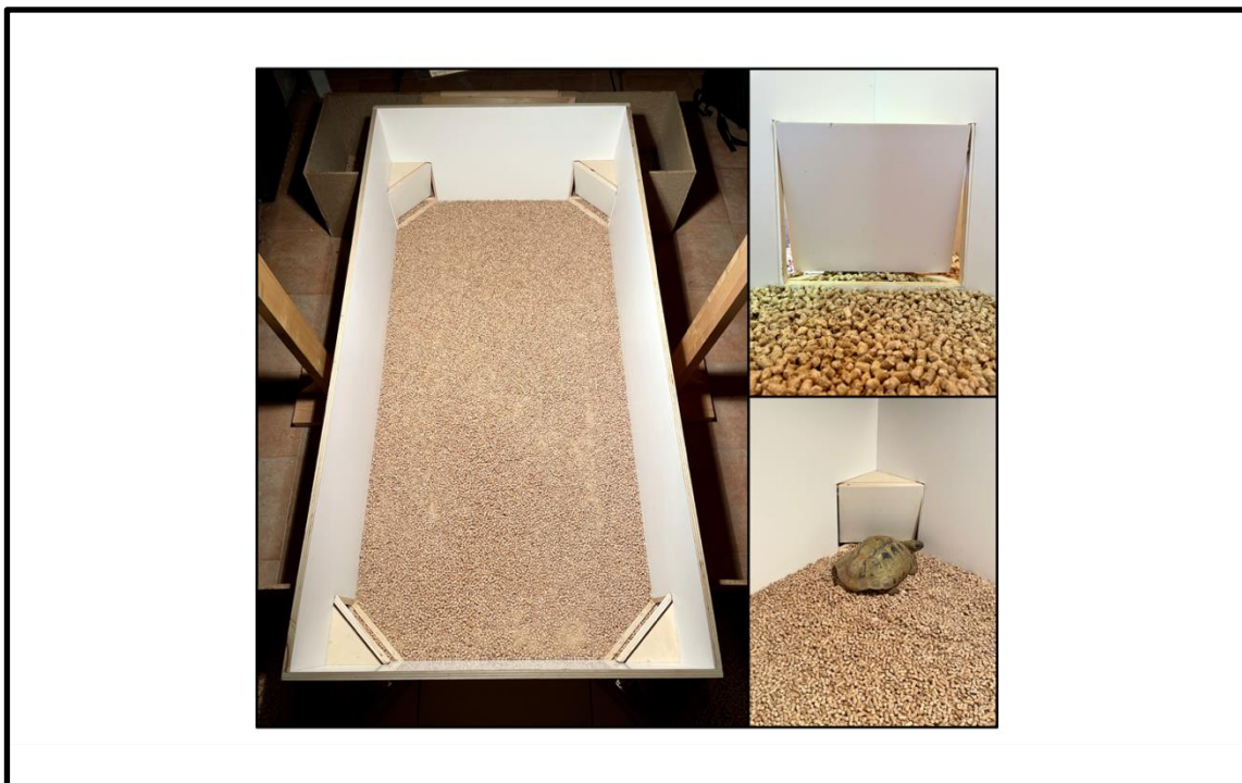
Figure 19. Photograph of the apparatus and detail of the up-and-over door. At the level of corners, the rectangular white arena had four holes supplied with doors that the tortoise could push to reach the external feeder box.
