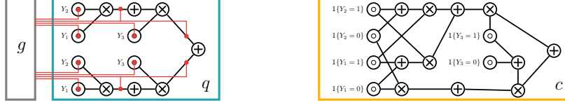
Figure 3: Examples of circuits in SPL. Left: a neural conditional probabilistic circuit q_{\Theta} . Red lines indicate how the output of g parameterizes the input distribution parameters \lambda and the sum unit parameters \omega of q , both indicated as red dots. Right: constraint circuit encoding the logical constraint of Eq. (1) where labels are Y_i \in \{Y_{\text{cat}}, Y_{\text{dog}}, Y_{\text{animal}}\} . Note that q and c are smooth, decomposable (Def. 3.3) and compatible (Def. 3.7) and c is deterministic (Def. 3.6). By parameterizing c via g we can obtain a single-circuit SPL (Sec. 3.4). Both: circuits q and c are compatible, as product units with the same scope decompose in the same way. E.g., consider the first two product units of q and c , right to left and top to bottom. Both units decompose \{Y_3, Y_2, Y_1\} into Y_3 and Y_2, Y_1 .
