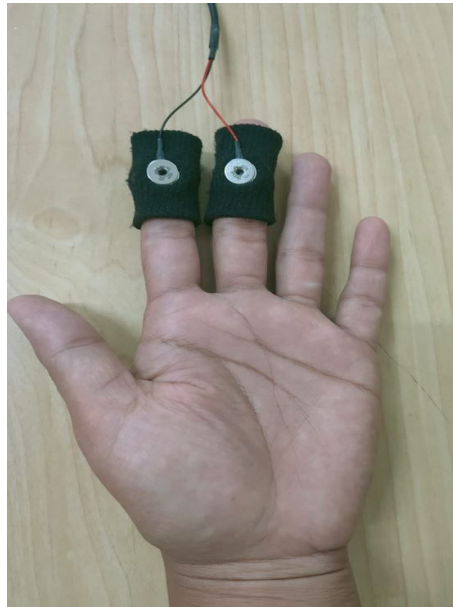
Figure 3.10: GSR sensor used for ET_Video_ES data collection
