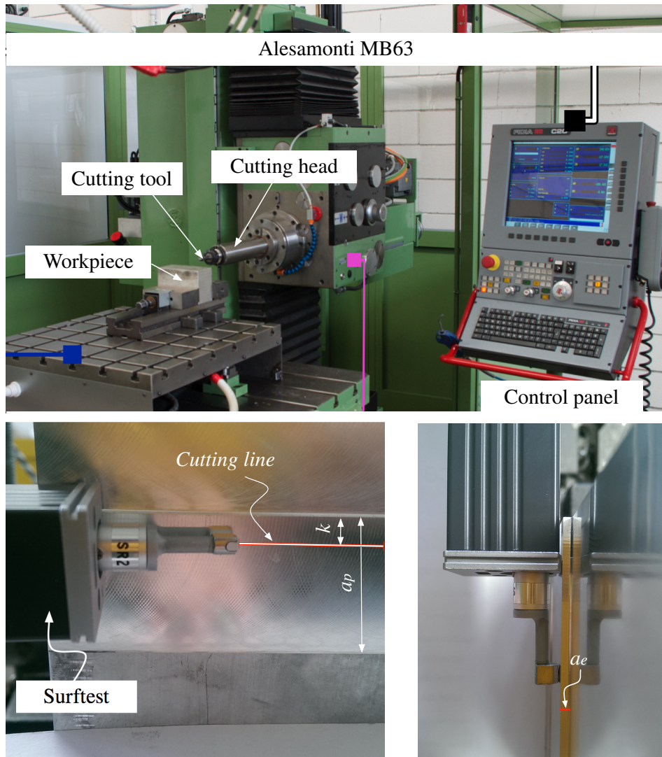
Figure 1.5: Experimental set-up: Alesamonti MB63 five-axis machining center; 63.0 mm diameter WIDIA M680 series end-mill; Mitutoyo profilometer SJ-210 series; a_p - axial cutting depth; a_e - radial cutting depth; k - distance at which a measuring line was selected
