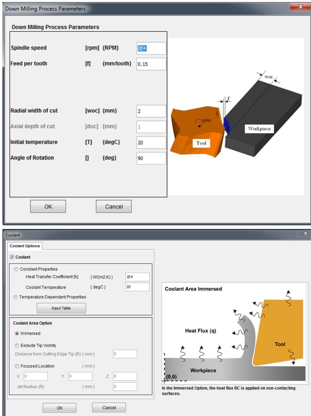
Figure 2.11: Example of the process set-up and default coolant properties in 3D FEM AdvantEdge [138]
