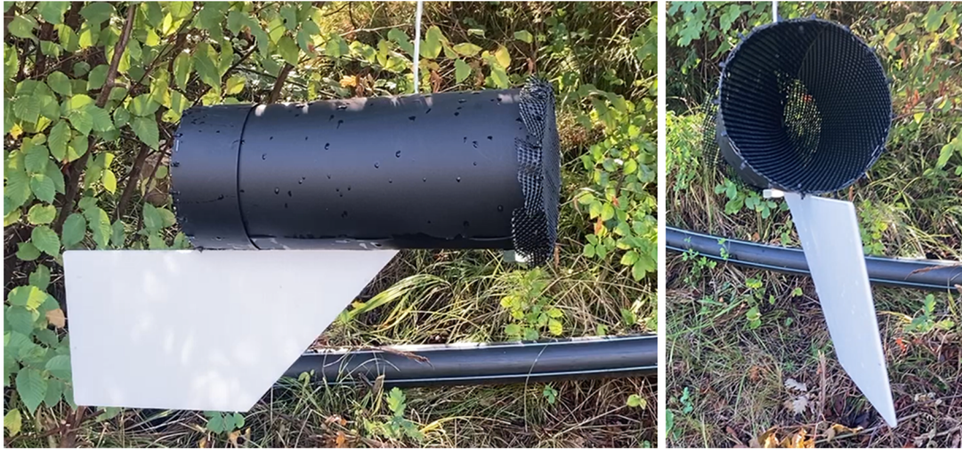
Fig. 1. A 150-mm diameter, 300-mm long wind-orienting tunnel trap prototype for Halyomorpha halys constructed of 1-mm thick polypropylene, Corflute windvane and 2-mm plastic mesh with a hex bolt counterweight. The right image shows the entry only mesh-cone.
