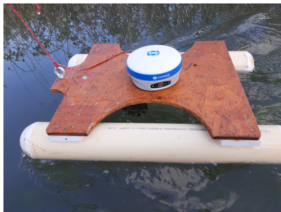
Figure 5.1: Float for bathymetric surveys with Deeper sonar and Stonex GNSS receiver
