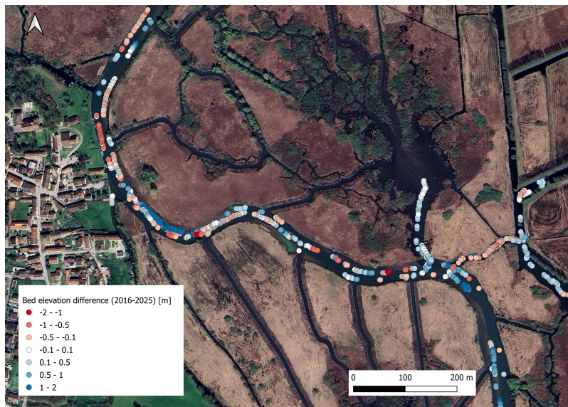
Figure 5.9: Bed elevation difference between 2016 and 2025 in the main Mincio River course near the village of Rivalta
