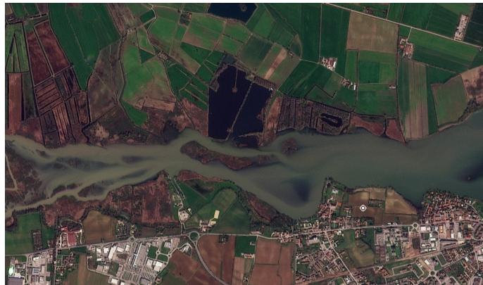
Figure 5.4: Planet satellite image of a sediment transport event (16 March 2025) showing high turbidity coming from upstream, with low interactions with the former quarry area
