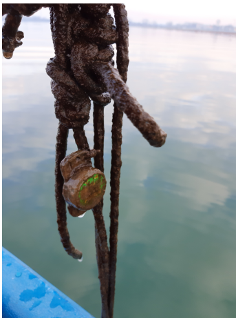
Figure 7.1: HOB0 temperature and light sensor after one month from the deployment
