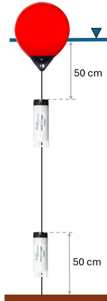
Figure 6.1: Schematic representation of the DO sensors' configuration
