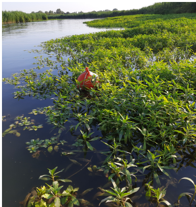
Figure 6.10: Picture of the buoy measuring dissolved oxygen inside the Ludwigia mat
