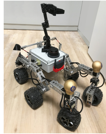
Fig. 2: Prototype of the UGV platform with a modular active sensing payload
