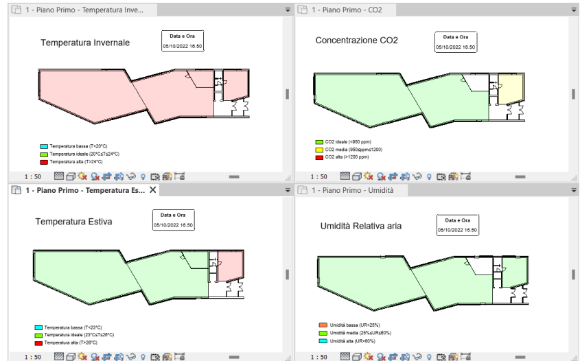
Figure 5.7 - Sensor data visualisation through Heritage Building Information Model (Murer, 2023).
