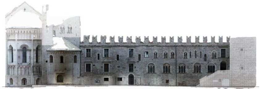
Figure 3.1 - West façade photogrammetric reconstruction of Palazzo Pretorio in Trento showing an example of complex and stratified heritage of building. Elaborations by LAMARC.
