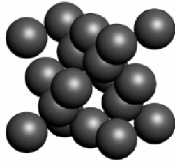
Fig. 2. The diamond lattice that was the first that presented a complete photonic band gap.
