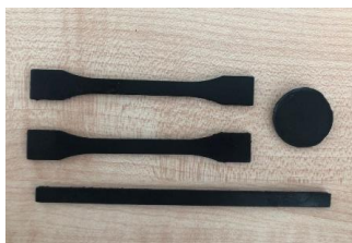
Figure 3-3: Compression molded samples used for different tests.
