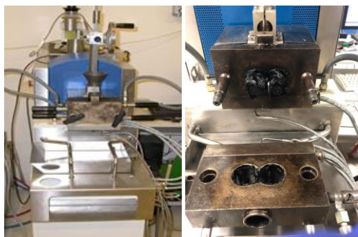
Figure 3-1: Photographs of Haake® internal mixer and mixing chamber.
