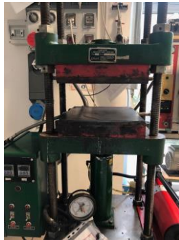
Figure 3-2: Carver® laboratory hot plates press.
