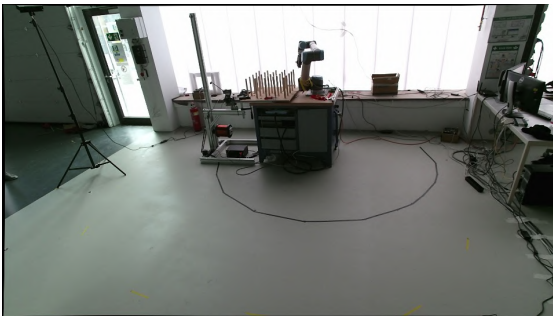
Figure 7. Experimental testbed in Stuttgart. The black tape on the floor represent the danger zone, with the robot manipulator at its center.
