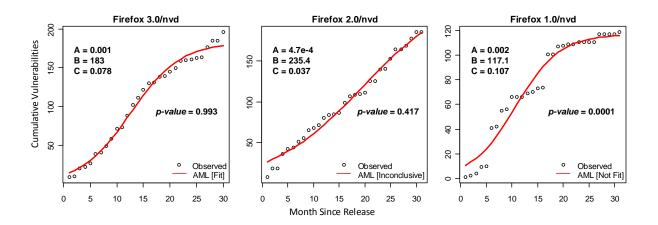
A,B,C are three parameters in the formula of the AML model:  $\Omega(t) = \frac{B}{BCe^{-ABt}+1}$  (see also Table 7.2)
