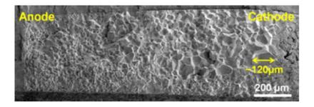
Figure 14: SEM micrograph on a 8YSZ flash sintered specimen showing a strong microstructure asymmetry (24 h at 1250°C, 50 A/cm<sup>2</sup>). Taken from [49].
