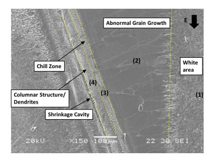
Figure 38: SEM micrograph of the blackened areas obtained on a sample treated with 7 mA/mm2 for ~ 4 minutes (experimental set up 2). The micrograph was taken in the central part of the gage section. The field direction is indicated by the black arrow; the different microstructural areas are indicated and numbered.
