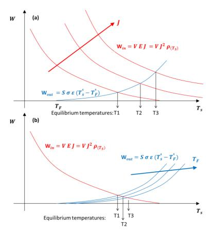
Figure 32: Current (a) and furnace temperature (b) effect on the equilibrium sample temperature during the steady state of FS. The equilibrium temperature is reached when the electrical power is equal to the heat exchanged by radiation. One should also remember that the onset for FS is depending from the field strength, resulting the specimens treated with higher E sintered at a lower furnace temperature.
