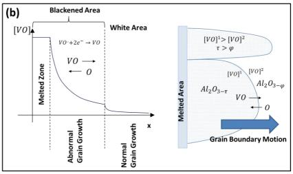
Figure 41: Possible mechanisms at the base of abnormal/anisotropic grain growth at the interface between blackened and white areas (a) and within the blackened one (b). The mechanism (a) is based on the assumption that the abnormal grain growth is associated to the growth of the substoichiometric phase. The mechanism (b) assumes the presence of a discharged vacancy gradient in the blackened areas which accelerate the mass flux.
