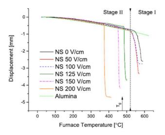
Figure 18: Electric field-induced softening in a sodium-silicate glass using different field strength. Taken from [119].
