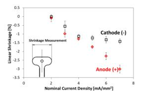
Figure 36: Linear shrinkage achieved in the electrode area (experimental set up 2, pre-sintering temperature = 1250 °C, E= 750 V/cm).
