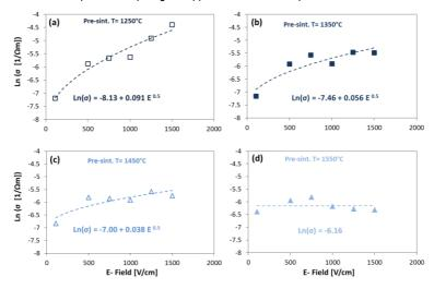
Figure 50: Conductivity for samples pre sintered at different temperature as a function of the field strength; the dashes lines represent the interpolation given by the Poole-Frenkel model. The data are referred to the very beginning of the incubation stage of flash sintering, when the power supply was turned on (Ts  $\sim$  Tf =1200°C). Modified from [16].
