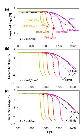
Figure 25: Dilatometric curves obtained using different fields (250 - 1500 V/cm) and nominal current limits of 2 (a), 4( b) and 6 mA/mm<sup>2</sup> (c). Modified from [55]. Modified from [55].
