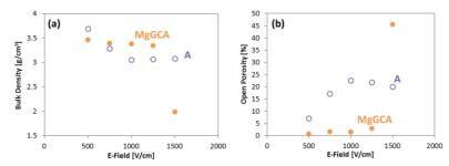
Figure 55: Bulk density (a) and open porosity (b) values measured on A and 10 wt% MgGCA samples flash sintered using different fields and a current limit of 2 mA/mm<sup>2</sup> (current limit maintained for 2 min). Modified form [187].
