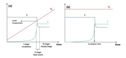
Figure 5: Electric field (E) and current (J) evolution during constant heating rate (a) and constant furnace temperature, Tf, (b) flash sintering experiments.
