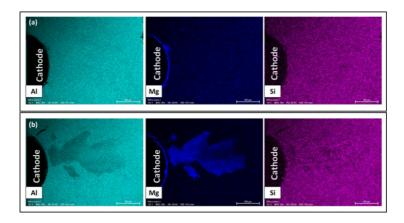
Figure 67: EDS concentration maps for Al, Mg and Si in the cathodic area of a MgGCA sample treated with 2 mA/mm2 under 500 (a) and 1000V/cm (b). Taken form [187].
