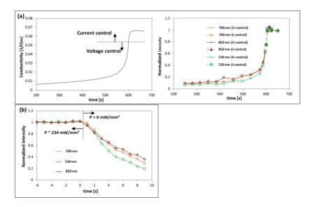
Figure 45: Normalized light emission evolution at different wavelength during the incubation (a) of FS and after the power supply was switched off (b). It is also reported the conductivity evolution which can be well compared with light emission.
