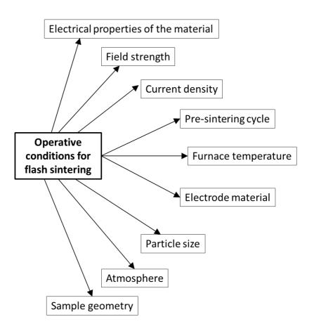
Figure 4: Process parameters that influence the flash sintering behavior.
