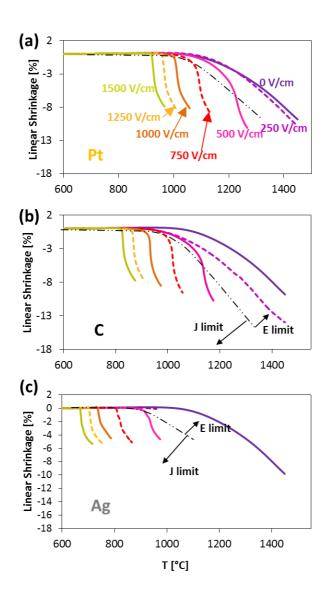
Figure 51: Dilatometric plots for samples treated using a current limit of 2 mA/mm^2 and different electrode materials: platinum (a), carbon (b) and silver (c).
