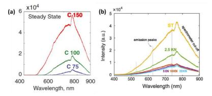
Figure 16: UV/VIS photoemission spectra obtained on YSZ using different current limit (a)[18] and on strontium titanate, potassium niobate and teir composites (b) [20].
