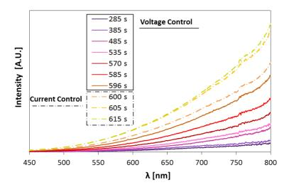
Figure 44: UV/VIS photoemission spectra obtained during the different stages of FS.
