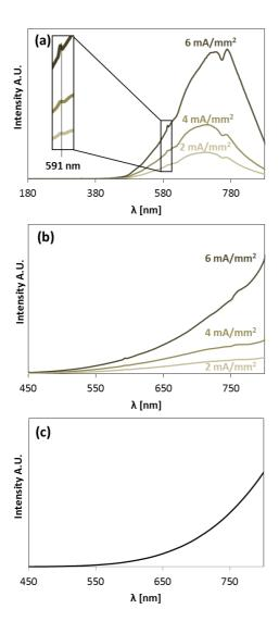
Figure 43: Photoemission spectra collected during the steady stage of flash sintering using different current density (samples pre-sintered at 1250°C). In particular are reported both the spectra as collected (a) and after the calibration with halogen lamp (b). For comparison the black body spectrum, calculated at 1600 K, is also reported (c).
