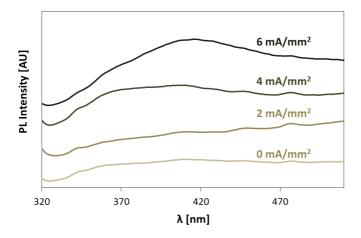
Figure 34: Phololuminescence spectroscopy of alumina samples treated with different current density.
