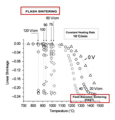
Figure 21: FS and FAST regime in YSZ upon constant heating rate experiments (10°C/min). Modified from [6].
