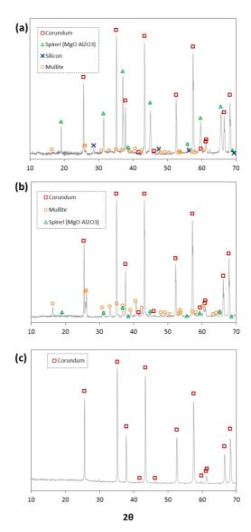
Figure 68: XRD spectra collected on the cathode (a), anode (b) and center of the gage section (c) on a MgGCA sample treated using 1000 V/cm and 2  $mA/mm^2$ .
