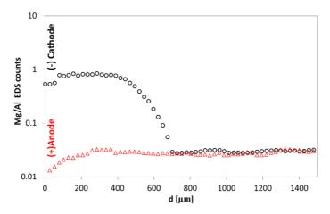
Figure 66: Ratio between magnesium and aluminum EDS counts at different distances from the cathode (black circles) and anode (red triangles) in a MGGCA sample treated with 750V/cm and 2 mA/mm<sup>2</sup>. Modified form [187].
