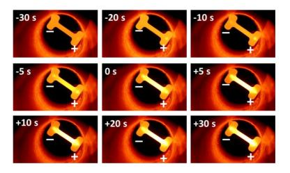
Figure 35: Pictures of a sample subjected to flash sintering at different times (t = 0 s was assumed to correspond to the system reaching the current limit).
