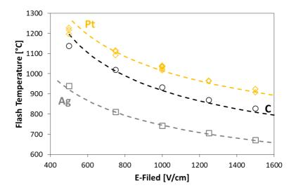
Figure 52: Onset temperature for FS as a function of the applied field strength for different electrode materials. Modified from [55].
