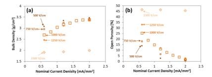
Figure 56: Bulk density (a) and open porosity (b) as a function of the current density for 10 wt% MgGCA specimens. Green density ~ 1.76 g/cm<sup>3</sup>, current limit maintained for 2 min. Modified form [187].
