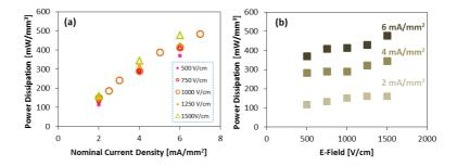
Figure 31: Specific power dissipation measured during the steady state of flash sintering as a function of the nominal current density (a) and of the E-field (b). Modified from [55].
