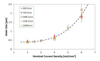
Figure 28: Grain size evolution as a function of the nominal current density, the dark-blue dashes line represent the fitting given by Eq.17.
