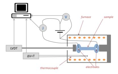
Figure 23: Experimental set-up for constant heating rate experiments.
