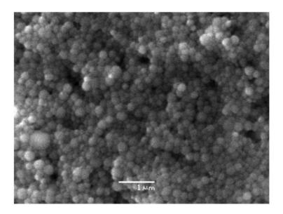
Figure 13: SEM micrograph of a dense flash sintered GDC specimen with sub-micrometric grain size. Taken from [34].
