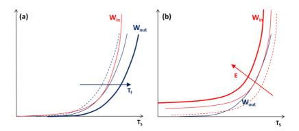
Figure 6: Flash sintering onset determination for constant heating rate (a) and isothermal flash sintering experiments (b). The dashes lines represent condition where FS cannot be reproduced, the thin continous lines are the onset for FS, the thik continous lines are conditions leading to the flash.
