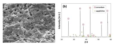
Figure 60: SEM micrograph (a) and XRD pattern (b) of a MgGCA specimen treated at 1350°C for 2 h. Modified form [187].
