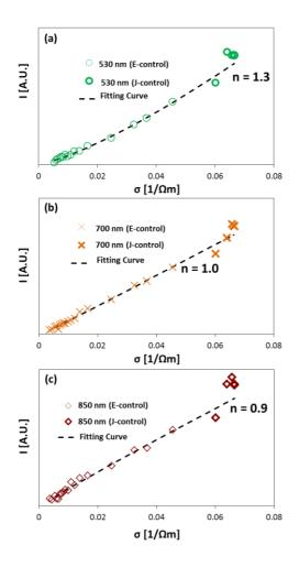
Figure 46: Light emission intensity as a function of the measured conductivity at different wavelength: 530 (a), 700 (b), 850 nm (c). The value of n, the exponent of the fitting power law, is also reported.
