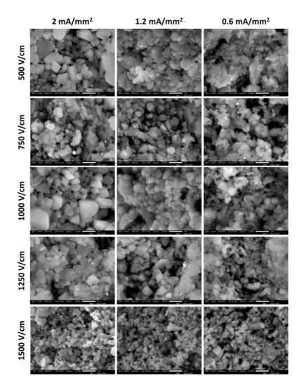
Figure 59: SEM micrographs of HF etched sample (MgGCA) treated using different combination of E and J (the inter-granular porosity is opened by the etching process). Modified form [187].
