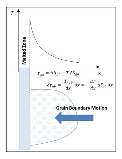
Figure 42: Mechanism for oriented grain growth in the blackened areas based on a thermal gradient. The grain boundary would migrate toward the hotter region (melted zone) as a result of a net decrease in the grain boundary energy ( $\delta\gamma_{ab}$ ).
