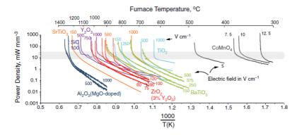
Figure 15: Power dissipation as a function of the inverse of furnace temperature for different materials. The furnace heating rate was 10°C/min and the sample geometry was dog bone-like, the span between electrode was 20 mm and the cross section approximately 3x 1.6 mm<sup>2</sup>. Taken from [88].
