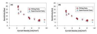
Figure 33: Resistivity calculated during the third stage of FS from electrical and geometrical parameters without (a) and with taking in account of the effect of porosity (b). The best interpolation was given using: Q = 0.94 eV,  $\epsilon = 0.65$  (a) and Q = 0.76 eV,  $\epsilon = 0.60$  (b). Modified from [55].
