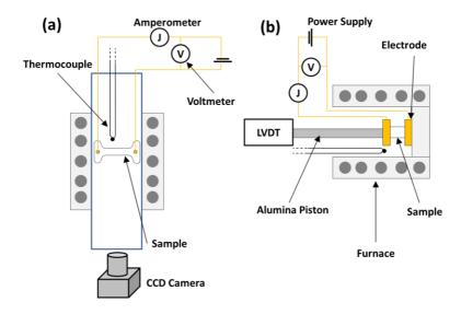
Figure 2: Two possible experimental set up for flash sintering experiments: the sintering can be monitored by a CCD camera (a) or by an LVDT sensor (b).
