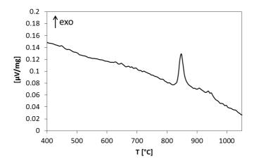
Figure 63: DSC of MgGCA powder (heating rate = 20°C/min).
