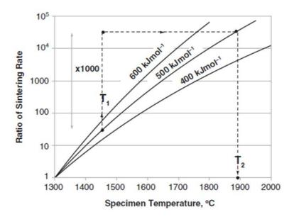
Figure 11: Sintering rate as a function of sample temperature using different activation energy for densification. T1 is the specimen temperature estimated using Eq.10; T2 is the temperature needed for justifying the observed sintering rates [65].
