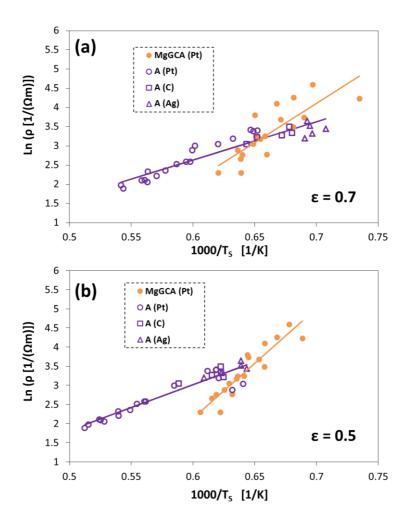
Figure 65: Electrical resistivity as a function of sample temperature for pure alumina and magnesia silicate glass-containing alumina assuming  $\epsilon$  = 0.5 (a) and 0.7 (b).
