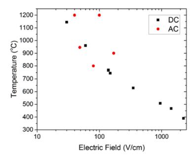
Figure 9: Relation between onset temperature for FS and applied field for 8YSZ in AC and DC treatments.[57]
