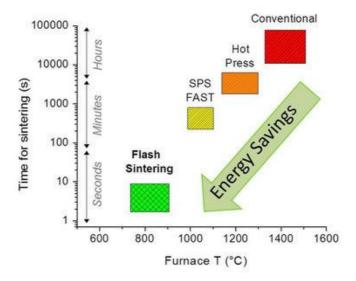
Figure 1: Typical time and temperature for sintering YSZ using different technologies. Taken from [10].
