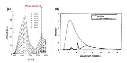
Figure 17: NIR light emission during flash sintering of 3YSZ (a)[17]; spectral emissivity of 13.5YSZ 1 mm thck single crystal (100) at 1000°C (b)[95].
