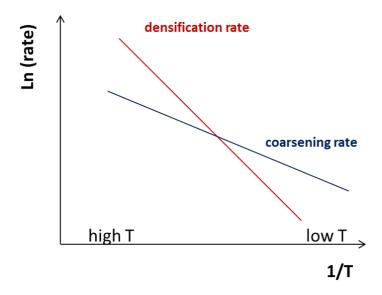
Figure 12: Qualitative behavior for sintering rate and grain coarsening under the assumption that the activation energy for the latter is lower. One can observe that at high temperature densification is enhanced, while at low temperature grain coarsening is more fast. In this case we assume that the sample temperature is homogeneous (grain boundary and grain core are at the same temperature).
