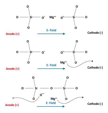
Figure 69: Structural rearrangement of glass structure during E-Field induced magnesium migration.
