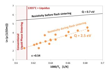
Figure 64: Resistivity during the third stage of FS as a function of the estimated sample temperature for MgGCA. One can observe that the behavior is different from what measured during the incubation of the process (black line). Modified form [187].
