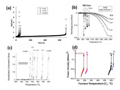
Figure 8: Sample length effect on incubation time for FS in Al<sub>2</sub>O<sub>3</sub>/YSZ composites (a)[56]. Effect of particle size (b)[62] and applied pressure on onset FS temperature for YSZ[63]. Onset temperature dependence from sintering atmosphere in ZnO (d) [64].
