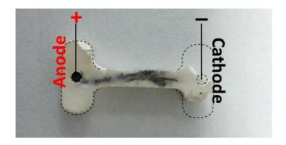
Figure 37: Blackened areas on a sample treated with 7 mA/mm<sup>2</sup> for ~ 4 minutes (experimental set up 2).
