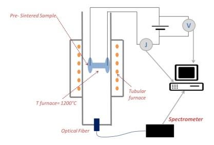
Figure 24: Experimental set-up for isothermal flash sintering experiments.
