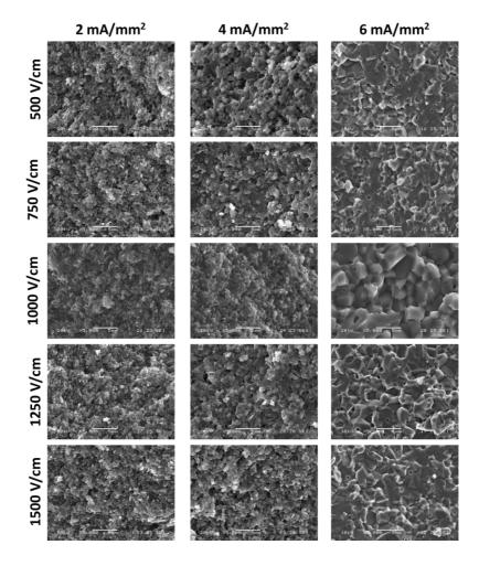
Figure 27: SEM micrographs of flash sintered sample using different combination of E and J.
