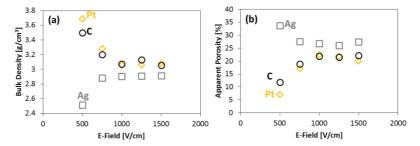
Figure 53: Bulk density (a) and apparent (b) of sample treated using different electrode materials and a current limit of 2 mA/mm<sup>2</sup>. Modified from [55].
