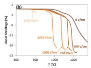
Figure 54: Dilatometric plots for pure alumina (a) and 10 wt% magnesia silicate glass-containing alumina (b) using different field strength and a current limit of 2 mA/mm $^2$ . Green density  $\sim$  1.76 g/cm $^3$ , current limit maintained for 2 min. Modified form [187].
