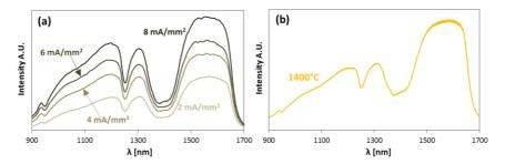
Figure 47: NIR spectra obtained during FS using different current density (furnace temperature= 1200°C) (a) and the thermal radiation of the furnace heated at 1400°C(b).
