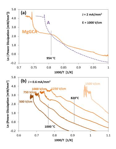
Figure 62: Comparison between specific power dissipattion in pure alumina and MgGCA (a) using 1000 V/cm and 2 mA/mm<sup>2</sup>. The effect of the field strength on the power dissipation of MgGCA is also reported (b). Modified form [187].
