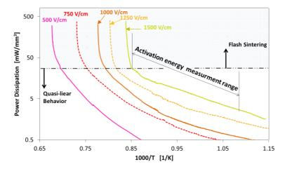
Figure 30: Natural logarithm of the specific power dissipation during the incubation of FS as a function of the inverse of the absolute furnace temperature (Pt electrodes, J = 6mA/mm<sup>2</sup>). Modified from [55].
