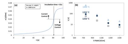
Figure 48: Conductivity evolution during the incubation of FS (a) and incubation time as a function of field strength and pre-sintering temperature (b). Modified from [16].
