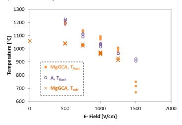
Figure 61: Onset temperature for flash sintering in MgGCA and A systems as a function of the field strength. The temperature at which the maximum shrinkage rate is reached during glass-softening (MgGCA) is also reported. Modified form [187].
