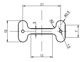
Figure 22: Specimen geometry used for flash sintering experiments (quote in mm).
