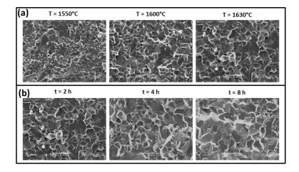
Figure 29: SEM micrographs on conventionally sintered specimens treated for 2 h at different temperatures (a) or at the same temperature (1630°C) for different times (b).
