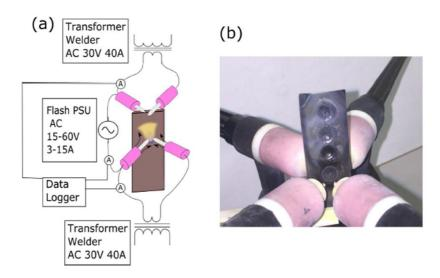
Figure 19: Experimental set-up for contactless flash sintering (a) and a picture of the used system (b). Taken from [114].
