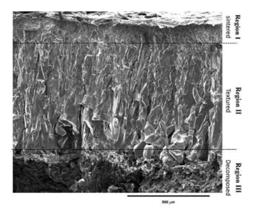
Figure 20: Textured SiC obtained by flash spark plasma sintering. Taken from [110].
