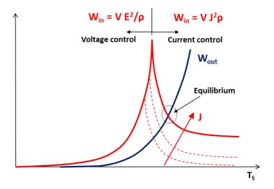
Figure 10: Qualitative power dissipation plot during the different stages of flash sintering.
