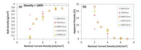
Figure 26: Density (a) and open porosity (b) evolution as a function of the nominal current density. Modified from [55].
