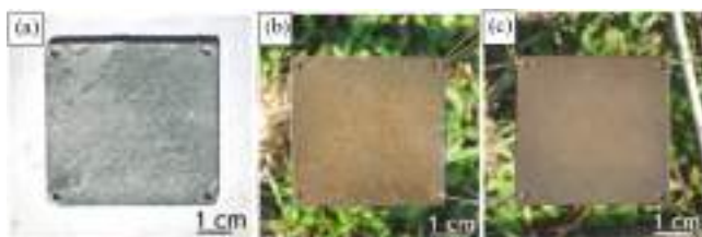
Fig. 9. (a) Bare, (b) PEO-coated, (c) PEO-coated and sealed AA2024 after 30 days of simulated marine exposure. Adapted from [28].
