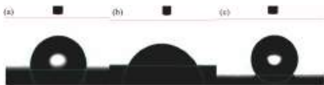
Fig. 17. Water Contact Angle on the surface of G16 alloy (analogous to AA2024) (a) uncoated, (b) PEO-coated, (c) PEO-coated with 2 g/L of graphene NPs. Adapted from [47].
