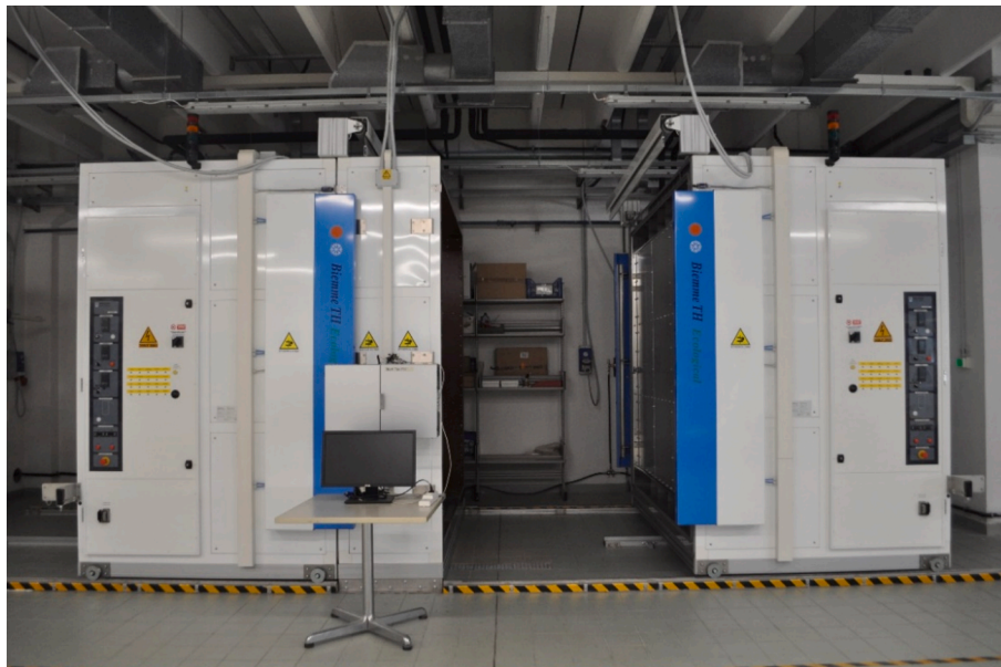
Fig. 2. Double climatic chamber at the Sustainable Energy Lab (University of Trento, Italy).
