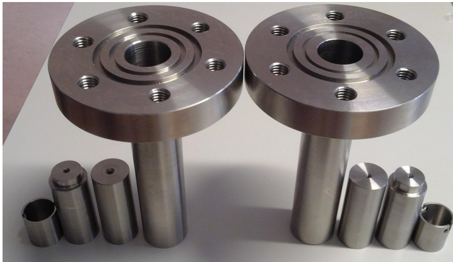
Figure 2.6: Bottom chamber for reference and sample side, with relative fillers and sample holder. A long unique fillers has been cut in two piece to facilitate the drilling of bottom piece.
