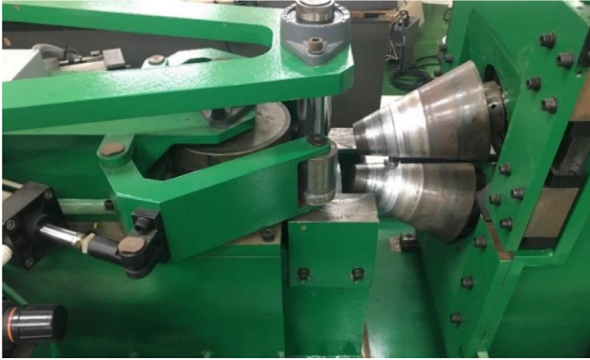
Fig. 13. Laboratory-size ring rolling machine utilized for the experiments.
