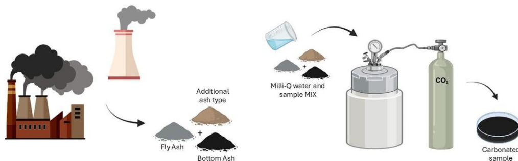
FIGURE 1 | Schematic representation of the accelerated carbonation process.
