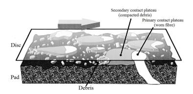
**Figure 4.4.1:** Schematic of the contact situation between an organic friction material and a brake disc and formation of compacted plateaus [source: Filip et al.,2002].
