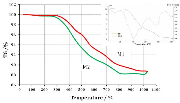
**Figure 8.3.1:** TGA curves of friction materials M1 & M2 in air. DTG curve of M2 in inset.
