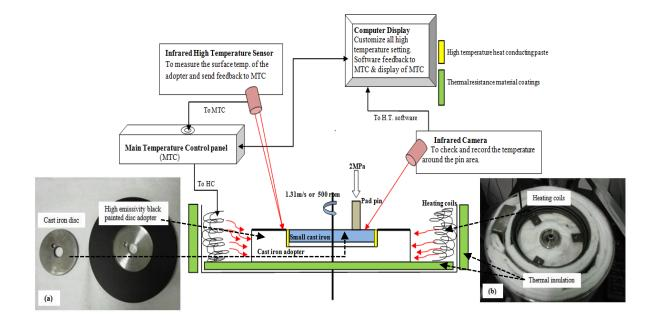
Figure 6.3.1: High temperature wear test rig.
