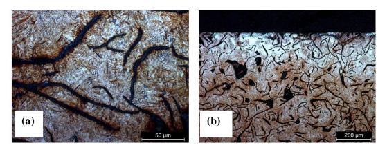
**Figure 8.4.1.** *a) Martensitic microstructure of heat treated disc, b) The decarburized surface of the heat treated disc.*
