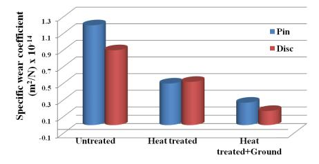
**Figure 8.4.4:** *Comparison of specific wear coefficient, K*<sub>*a*</sub>*, of the M2 pin and different discs.*
