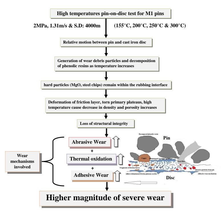
**Figure 8.3.16:** Wear mechanisms involved in dry sliding of M1 friction material at higher temperatures.
