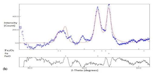
**Figure 8.2.3**: (a) Experimental imaging plate XRD ring pattern of stage\_12 of PC-M1. (b) Experimental (blue dots) and modelled (continuous black line) XRD spectrum patterns of stage\_12 of PC-M1. Main diffraction peaks of identified phases are marked in the graph.
