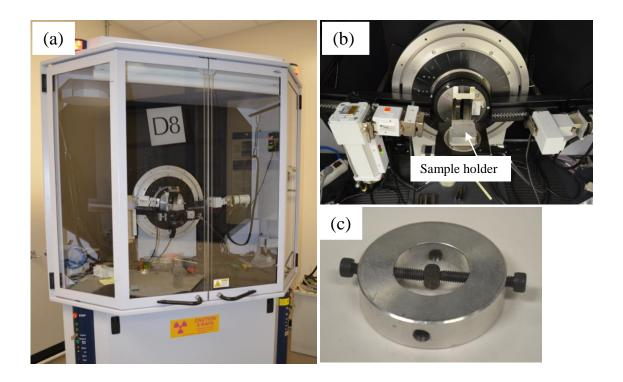
**Figure 7.4.6**: a) D8 diffractometer, b) position of sample holder, c) Sample holder with M1 pin.
