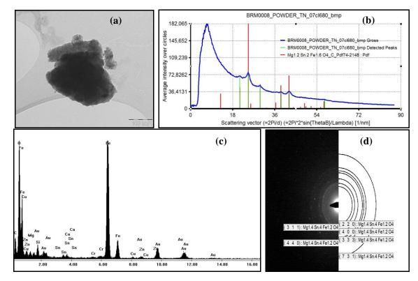
**Figure 8.1.7:** (a) Nano wear debris paricle of M1 brake material. (b) Process diffraction-identification of mixed phase of magnesium oxide, tin oxide and iron oxide as a major phases present in fig. 8.1.8a. (c) EDX analysis of fig. 8.1.8a M1 friction material wear debris. (d) Electron diffraction patterns (SAED) corresponding to nanocrystalline wear debris fig. 8.1.8a. The diffraction pattern shows concentric rings corresponding to Fe<sub>3</sub>O<sub>4</sub>, SnO<sub>2</sub> and MgO.
