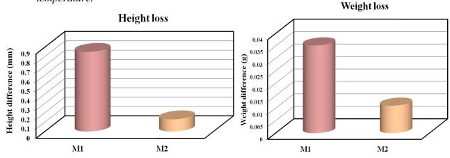
**Figure 8.1.2** : Shows the height loss difference and weight loss difference between the two friction materials: M1 & M2.
