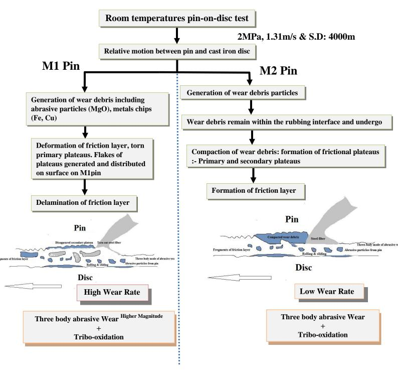
**Figure 8.1.11:** Wear mechanism involved in dry sliding of friction materials (M1 & M2) at room temperatures.
