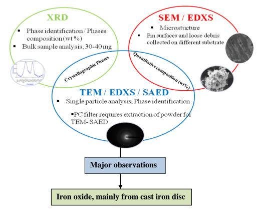
Figure 9.1.1: Reliable combination of characterization tools for particulate matters.
