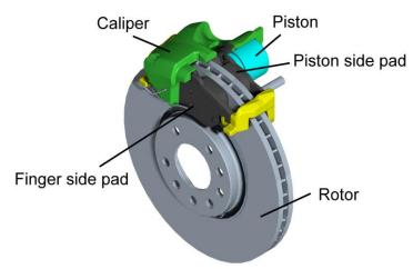
Figure 2.2.1: Schematic diagram of disc brake system. [Source: Jens wahlstrom et al, 2009].
