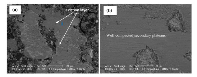
**Figure 8.1.5**: *SEM images of the M2 pin worn surfaces rubbed against cast iron rotating disc.*
