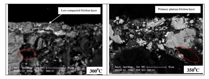
**Figure 8.3.10:** Cross section of worn pin surfaces of two friction materials M1 (a) & M2(b) at different temperatures.
