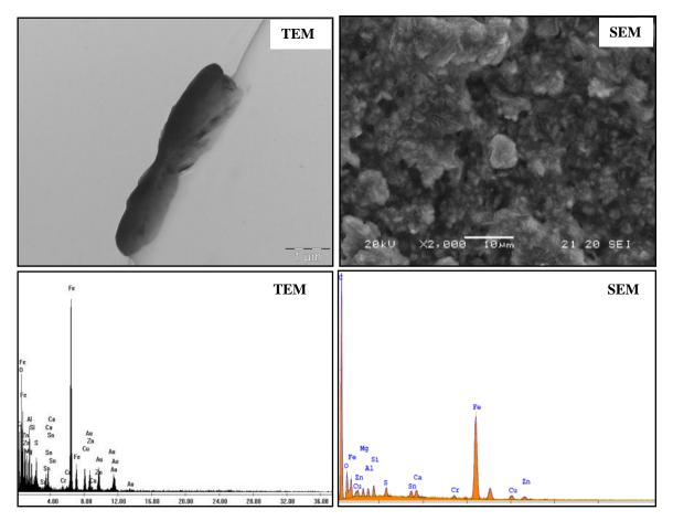
**Figure 8.2.15:** *PC-8 stage\_12 sample TEM (left) and SEM (right) wear debris and relevant EDX spectra. In both spectra the main detected elements are indicated. Gold lines in EDXS-TEM spectrum are due to carbon coated gold grid used for TEM sample preparation.*
