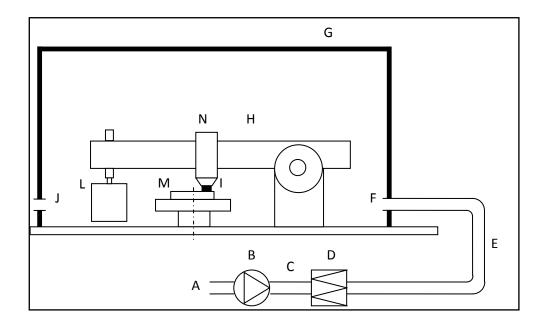
**Figure 7.3.2**: Schematic of the test equipment [Olofsson et al.,2009]. A: Room air; B: Fan; C: Flow rate measurement; D: Filter; E: Flexible tube; F: Inlet for clean air, measurement point; G: Closed box (Chamber); H: Pin-on-disc machine; N: Air inside box, well mixed; J: Air outlet, measurement points; L: Dead weight; M: Rotating disc sample; I: Pin Sample.
