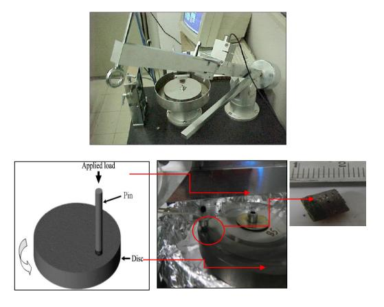
Figure 7.3.4: Pin-on-disc equipment with aluminum foil for collecting of wear debris.
