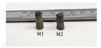
Figure 7.1.1: Brake pad pins from the two different friction materials, M1 & M2.
