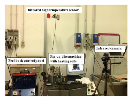
**Figure 7.3.5:** *Real time and schematic closed loop feedback high temperature wear test setup.*
