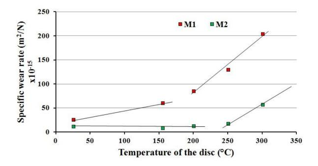
**Figure 8.3.3:** Specific wear behaviour of M1 & M2 friction materials pin at different temperatures.
