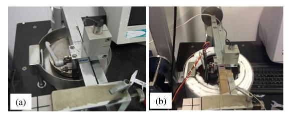
**Figure 7.3.6: a)** Low temperature Pin-on-disc: Frictional heating system with 140mm diameter cast iron disc used in Case I. b) High Temperature Pin-on-disc: External heating system with 63.0 mm diameter cast iron disc used in Case III.
