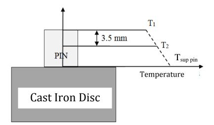
Figure 7.3.11: Diagram showing  $T_{sup}$  which is resultant linear gradient of T1 and T2.
