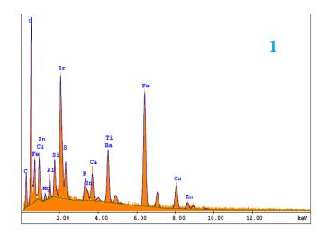
**Figure 8.1.6**: (a) Energy dispersive X-ray spectroscopy analysis of the third layer formed on the worn surface of M2 pin when tested against rotating cast iron disc.
