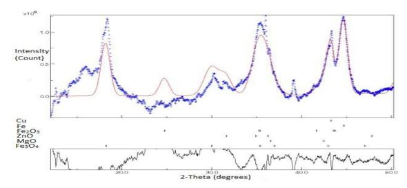
**Figure 8.2.2**: *Experimental (blue dots) and modelled (continuous black line) XRD spectrum patterns of AF-M1 sample. Main diffraction peaks of identified phases are marked in the graph.*
