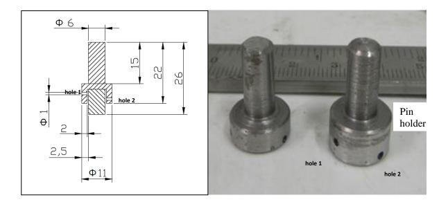
Figure 7.3.10: Pin holder with two holes for chromel-alumel-type thermocouples.
