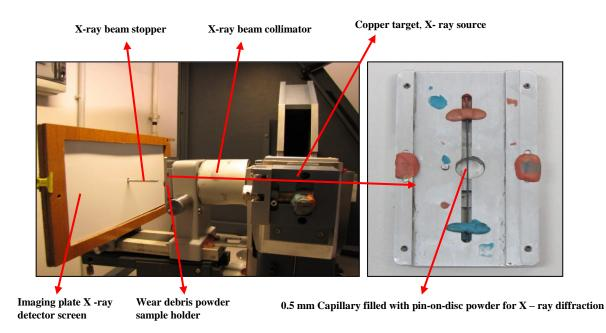
Figure 7.4.2: IPD 3000 Diffractometer: transmission mode configuration.
