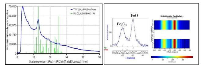
**Figure 8.2.13:** SAED (left) and XRD (right) patterns for PC-M1 stage\_12 sample. In the SAED in green reference lines for  $Fe_2O_3$ . As concerns the XRD pattern, the main diffraction peaks of identified phases are marked.
