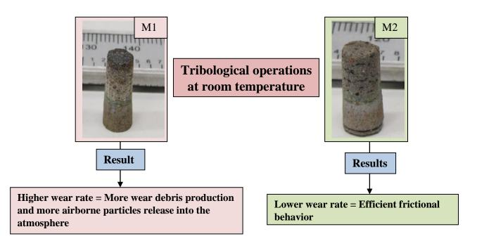
Figure 6.1.1: The flow-chart of tribological results of M1 & M2 friction materials.
