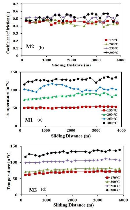
**Figure 8.3.2:** Evolution of the friction coefficient of M1 & M2 friction materials (a & b) and (c & d) extrapolated contact temperature of pins measured by thermocouple at 6mm and at 4mm.
