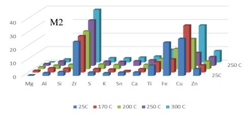
Figure 8.3.11: Average elemental composition of friction layer on M2 cross section surfaces.
