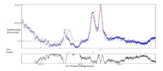
**Figure 8.2.4:** *Experimental (blue dots) and modelled (continuous black line) XRD spectrum patterns of stage\_15 of PC-M1 sample. Main diffraction peaks of identified phases are marked in the graph.*
