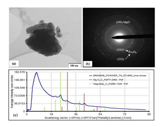
**Figure 8.2.11:** *TEM image (a) and relevant SAED of sample AF-M1. (c) Process Diffraction analysis of the same SAED pattern showing the imaged particles contain iron (red) and magnesium (green) oxides.*
