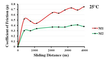
**Figure 8.1.1**: *Coefficient of friction vs sliding distance of M1 & M2 at 25°C temperature.*
