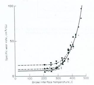
**Figure 4.4.2:** *Influence of contact temperature on the wear rate of a friction material [Source: A.E. Anderson et al., 1992, wear control handbook].*
