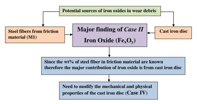
Figure 6.4.1: *Highlighting the reason for the heat treatment of the cast iron disc.*
