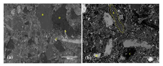
**Figure 7.1.2:** *Microstructure of virgin friction materials (a) M1 friction material in which A: Steel fiber, B: Magnesium oxide , C:Tin sulfide and D: Area rich in Fe, Mg, Ca and Zn. (b) M2 friction material where A: Potassium titanate fibre, B: Tin sulfide and C: Resin binder.*
