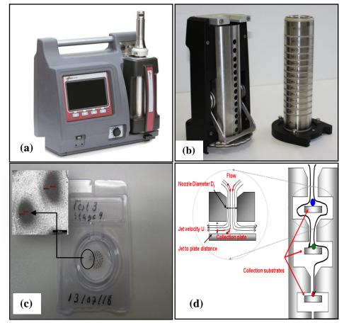
**Figure 7.3.3:** *ELPI*+ particle collection instrument (a) and (b). Polycarbonate filters with collected particles, (c). Scheme of working principles, (d).
