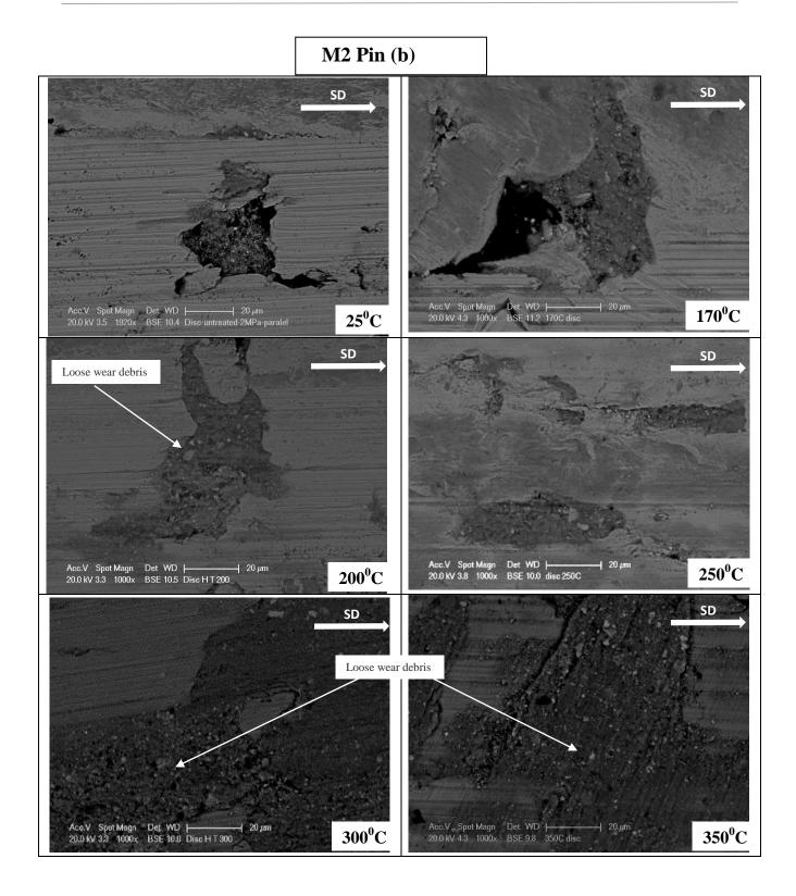
Figure 8.3.8: SEM observation of disc surface of M1 (a) and M2(b) at different temperatures.
