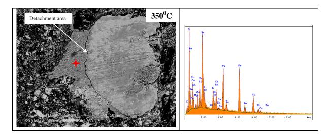
**Figure 8.3.4:** SEM of worn surfaces of M1 (a) & M2 (b) friction materials pins at different elevated temperature.
