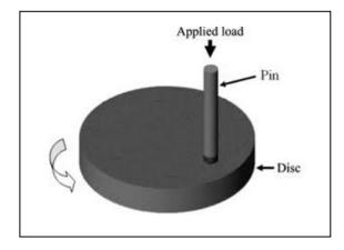
Figure 7.3.1: Simple pin-on-disc machine fundamentals.
