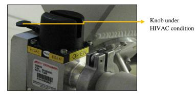
**Figure 7.4.9:** *Switching valve for high vacuum (HV) or low vacuum (LV=ESEM) SEM operational modes.*
