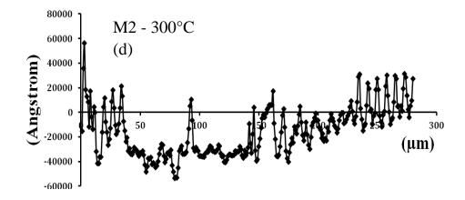
**Figure 8.3.9:** Average elemental composition of wear debris on M1(a) & M2(b) disc surface respectively.(c) & (d) profilometry profile of worn cast iron disc of M2 at different temperatures.
