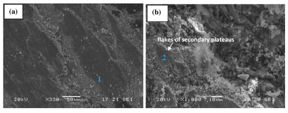
Figure 8.1.3: SEM images of the M1 pin worn surfaces rubbed against cast iron rotating disc.
