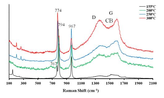
**Figure 8.3.14**: Comparison of Raman spectroscopy at secondary plateaus of a worn pin surface under different working temperature.
