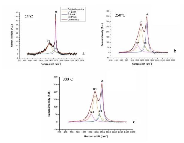
**Figure 8.3.7:**(*a*) Lorentzian curve fit for the deconvoluted Raman spectra of black carbonaceous product of high temperature frictional test at 25°C, (b) 250°C and (c) 300°C.
