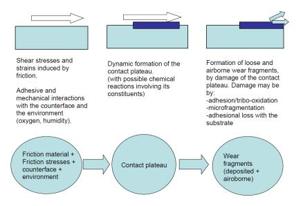
Figure 4.4.4: Summary of the basic wear mechanisms in braking systems.
