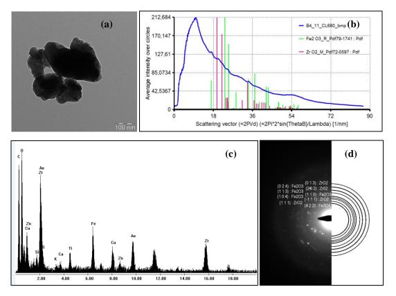
**Figure 8.1.9**: (a) Nano wear debris paricle of M2 brake material. (b) Process diffraction – identification of iron oxide and zirconium oxide as a major phases present in fig. 8.1.6a. (c) EDX analysis of fig.8.1.6a M2 friction material wear debris. (d) Electron diffraction patterns (SAED) corresponding to nanocrystalline wear debris fig.8.1.6a. The diffraction pattern shows concentric rings corresponding to  $Fe_2O_3$ ,  $Fe_3O_4$  and  $ZrO_2$ .
