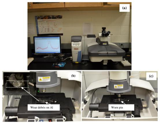
**Figure 7.4.11:** *a) A thermo scientific DXR Raman spectrometer, b) wear debris Raman analysis, c) worn pin surface Raman analysis.*
