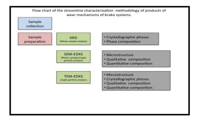
Figure 6.2.1: The flow-chart of the characterization methodology.
