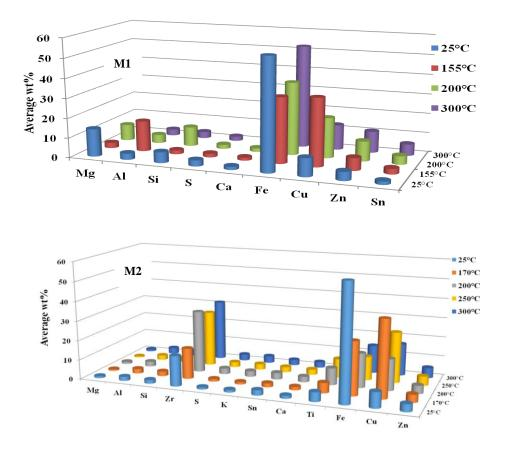
**Figure 8.3.5:** Average elemental composition of friction layer on M1 & M2 worn pin surfaceplanar view.
