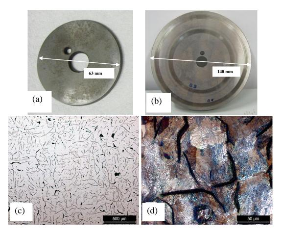
**Figure 7.2.1:** a) Optical image of the small cast iron disc, used in case III & IV b) Optical image of the big cast iron disc, used in case I & II, c)Microstructure of the grey cast iron, d) microstructure after etching with 2% Nital + 2% Picral (50-50 vol%).
