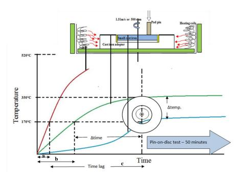
**Figure 7.3.8:** *Shows time lag of heating between the heating coils, adapter and cast iron disc.*
