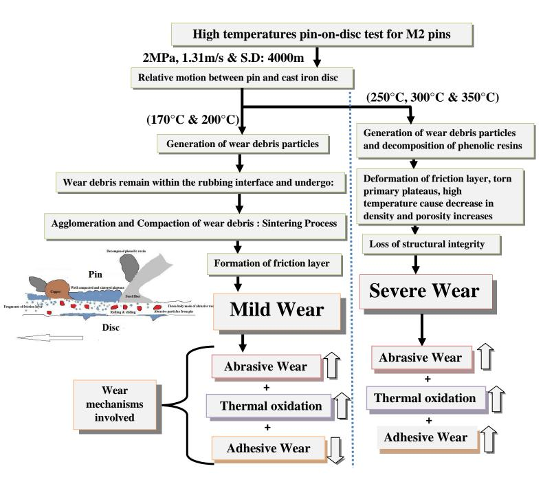
**Figure 8.3.15:** Wear mechanisms involved in dry sliding of M2 friction material at higher temperatures.
