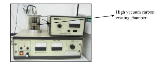
Figure 7.4.7: Carbon coating apparatus.
