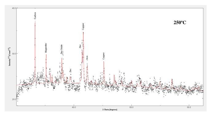
**Figure 8.3.13:** *Maud Rietveld fit relative to sample M1- 250°C with the identification of the most relevant phases.*
