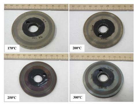
Figure 7.3.9: Tribo-oxidation of cast iron at different high temperature test.
