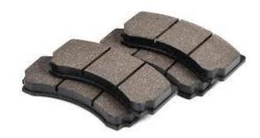
Figure 2.2.2: A commercial brake pad friction material.
