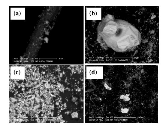
Figure 8.2.6: SEM images of pin-on-disc wear debris of AF-8.
