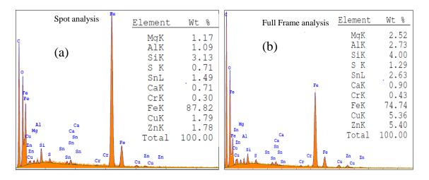
**Figure 8.2.7**: *EDAX spectrum (a) ultrafine particle of fig.8.2.6a, (b) full frame of coarser particles of fig.8.2.6c.*
