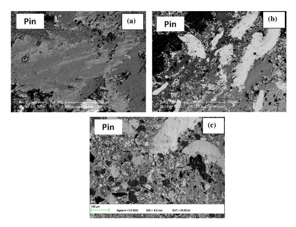
**Figure 8.4.5:** *SEM micrographs of the wear tracks on the pin surface after sliding against the untreated (a), the heat-treated (b) and the heat treated and grinded disc (c).*
