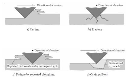
**Figure 4.3.1:** *Mechanisms of abrasive wear: microcutting, fracture, fatigue and grain pull-out [Source: Pooley et al., 1972].*
