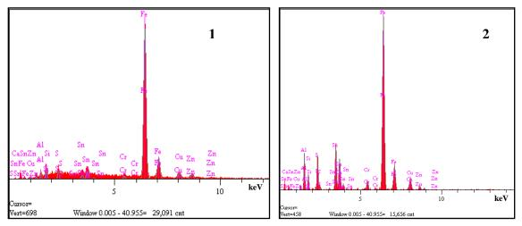
**Figure 8.1.4**:*Energy dispersive X-ray spectroscopy analysis of the third layer formed on the worn surface of M1 pin when tested against rotating cast iron disc at different location named 1 & 2 (see figures 8.1.5, a) and b)).*
