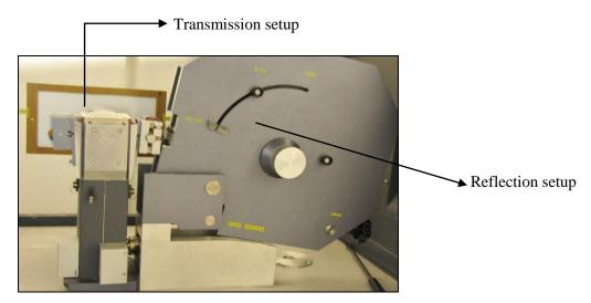
Figure 7.4.3: Two different configurations of operation for XRD analyses.
