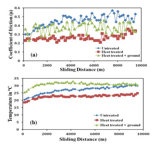
**Figure 8.4.2:** *Evolution of the friction coefficient (a) and of the average contact temperature (b) during wear tests.*
