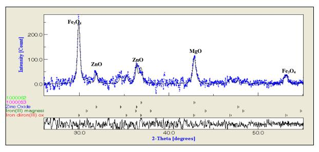
**Figure 8.1.8**: *X-ray diffraction of M1 wear debris powder (bulk) placed in a 0.5 mm capillary tube diffracted in transmission mode.*
