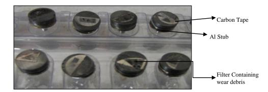
**Figure 7.4.8:** Carbon sputtered samples for SEM observation. In this case, a graphite disc substrate was also present on each SEM stub.
