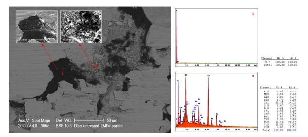
**Figure 8.4.6:** SEM planar view of the wear surface of the untreated cast iron disc. The picture shows a region where the graphite lamellae emerge (point 1) at the surface and there is an accumulation of wear fragments from the friction material (point 2) and corresponding EDX spectra of the highlighted regions.
