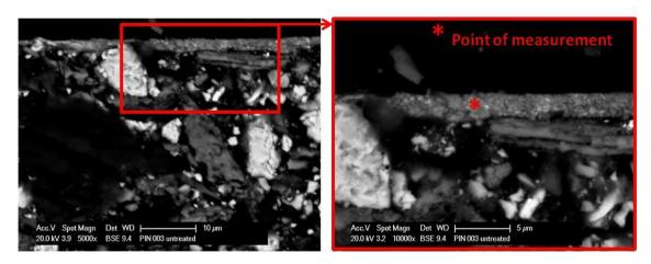
**Figure 8.4.7:** Cross sectional SEM micrographs of the friction layer on the pin after sliding against the untreated disc. Low (Sx) and higher (Dx) magnification.
