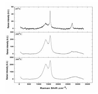
Figure 8.3.6: Raman spectra of decomposed phenolic resin at different temperatures.
