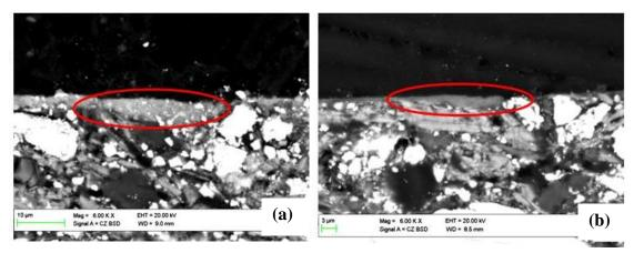
**Figure 8.4.8:** Cross sectional view of the pins against a) Heat treated, b) Heat treated and ground.
