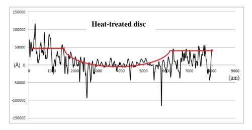
Figure 8.4.3: Surface profile across the wear track of heat treated disc.
