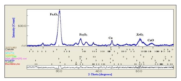
**Figure 8.1.10**: *X-ray diffraction of M2 wear debris powder (bulk) placed in a 0.5 mm capillary tube diffracted in transmitted mode.*
