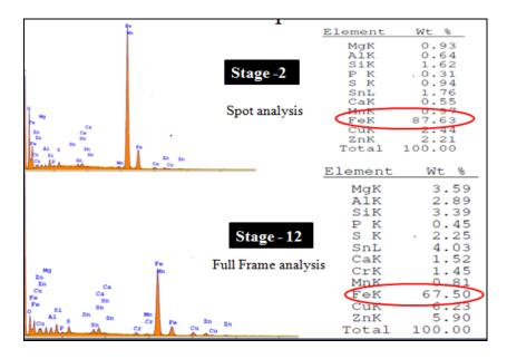
**Figure 8.2.9:** *EDAX spectrum (a) agglomerated particles of fig.8.2.8a, (b) full frame of coarser particles of fig.8.2.8e.*
