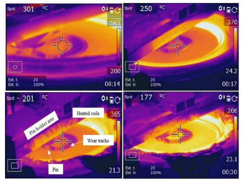
**Figure 7.3.7:** *Infrared camera images of high temperature pin-on-disc at different temperature.*
