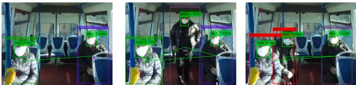
Fig. 19. Detection of users' face masks (FFP2 type) inside a vehicle of the PTS and social distance measurement.
