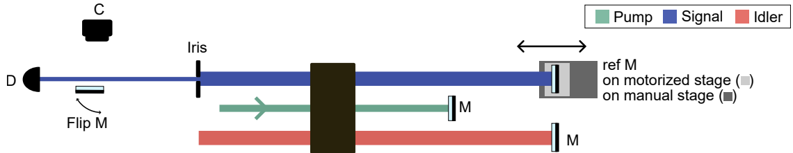
Figure 4.2.: Schematic of the experimental setup for measuring the interference visibility as a function of the reference signal mirror longitudinal coordinate. The position of the reference mirror (ref M) for the signal photons is controlled with a manual translational stage. At each position, the interference pattern in the signal modes is acquired with a single-pixel SPAD (D). To measure the interference pattern, the reference mirror is moved with a motorized stage. To access the single-pixel information, only a uniform region of the two-dimensional interference pattern is selected with an iris diaphragm (Iris). To verify that the iris is correctly centered, the signal beam is imaged on a camera (C) with a flip mirror (Flip M). The signal modes are coupled to the detector with an aspheric lens mounted on a micro-block stage (not pictured).
