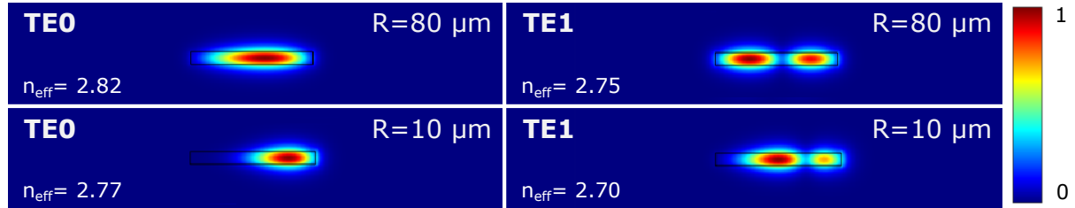
Figure 1.4.: Simulations of the normalized norm of the electric field for the fundamental and first-order TE optical modes at wavelength 1.55 \mu\text{m} in a bending waveguide, with bending radius R . Here is shown the cross-section of the curve, with the center of the curve located to the left. The waveguide core is made of silicon, and its cross-section is 2 \mu\text{m} \times 0.22 \mu\text{m} . The cladding is made of silica. The effective index is indicated for each mode with n_{\text{eff}} .
