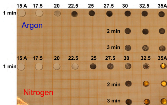
Fig. 6. Image of the samples under different current, time, and atmospheric (Ar and N_2 ) conditions.
