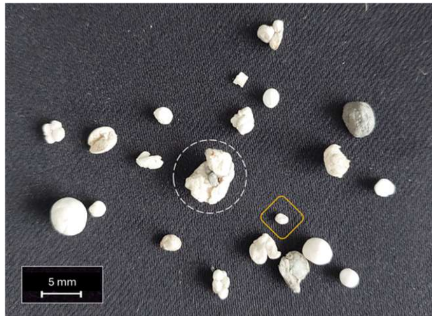
Figure 10. Optical image of 20 EPS microplastics from Sample W6 with average diameter of 3.3 \pm 1.1 mm, compared to an EPS mesoplastic of Sample W6 (evidenced by white dotted circle in the center). The orange diamond evidences the smallest EPS particle retrieved in Winter monitoring (ellipsoidal shape with axes of 1.5 and 1.9 mm; equivalent diameter of 1.7 mm).
