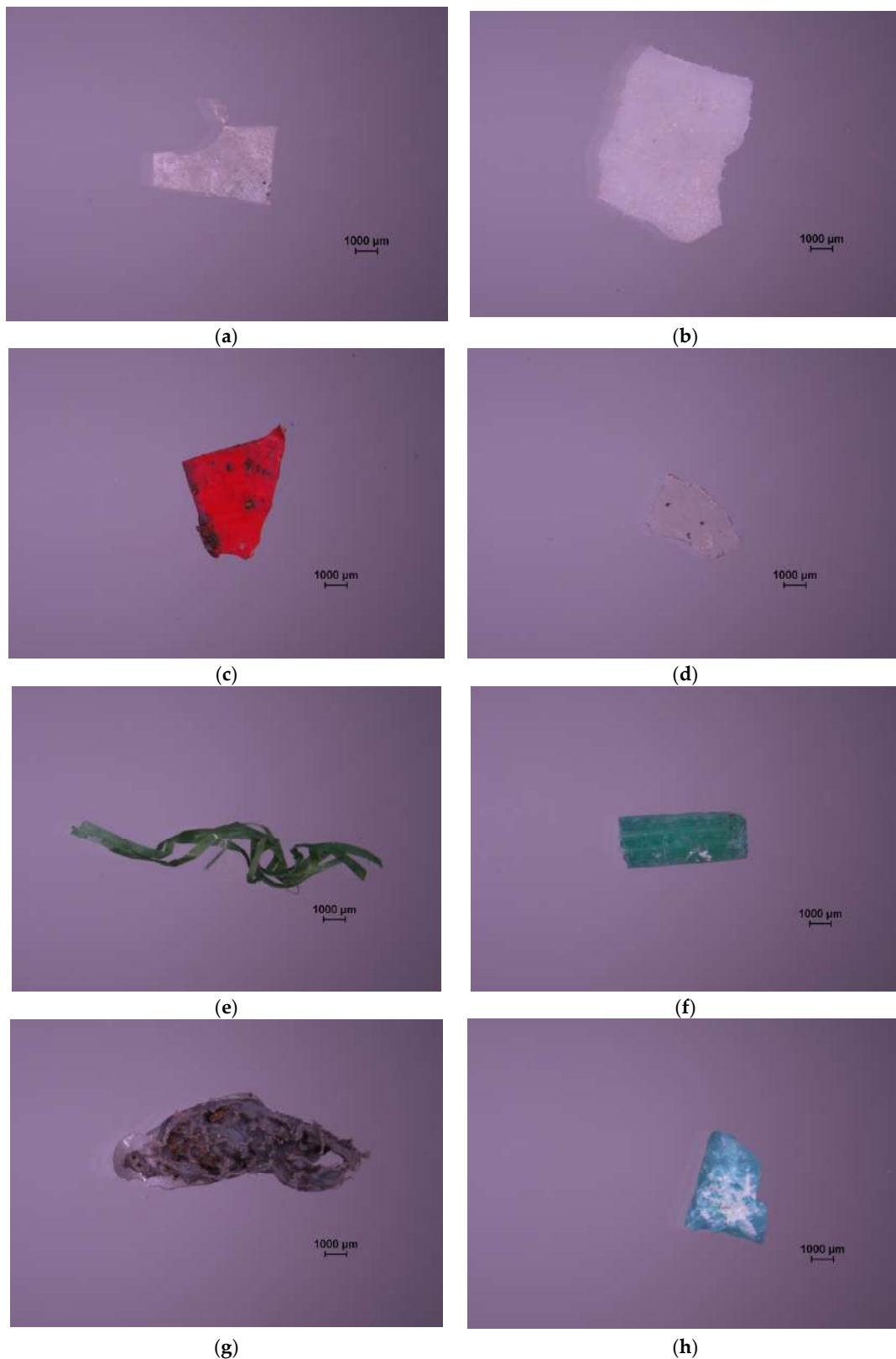
Figure A3. Representative PE microplastics of Sample W6 show different type of product. Film with average thickness of 0.23 \pm 0.04 micron (a–d); multifilament/stripe (e); fragments of IM products with average thickness of 1.4 \pm 0.4 mm (f–h). Specimen (g) shows contamination of inorganic matter. Average size of the PE specimens in Sample W6 is 2.3 \pm 0.7 mm, approximately calculated from the equation: size = \sqrt[3]{L \times W \times T} where L, W and T are the measured length, width and thickness of the specimen.
